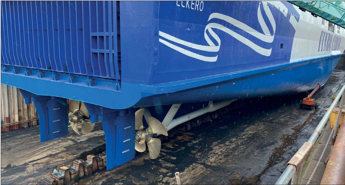
*Most of the underwater hull was coated with Ecospeed to make sure no repaint would be needed.*
