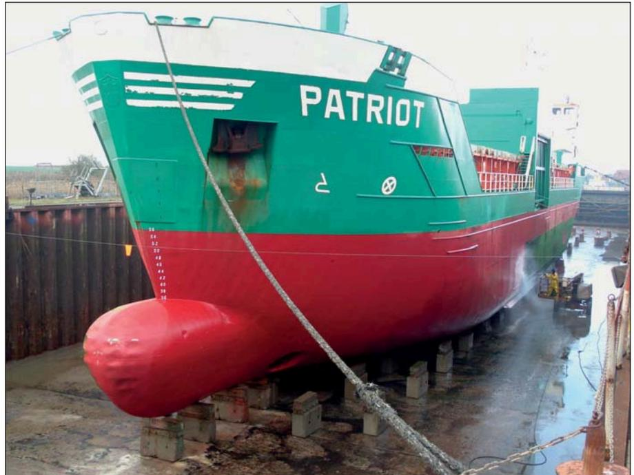
*Ecospeed can be easily cleaned in drydock or underwater without damaging the coating.*
