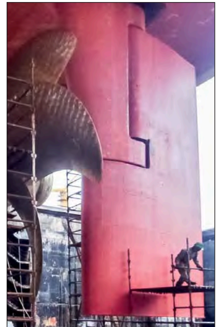
Rudder of m/v Deva after five years of service with Ecoshield.
