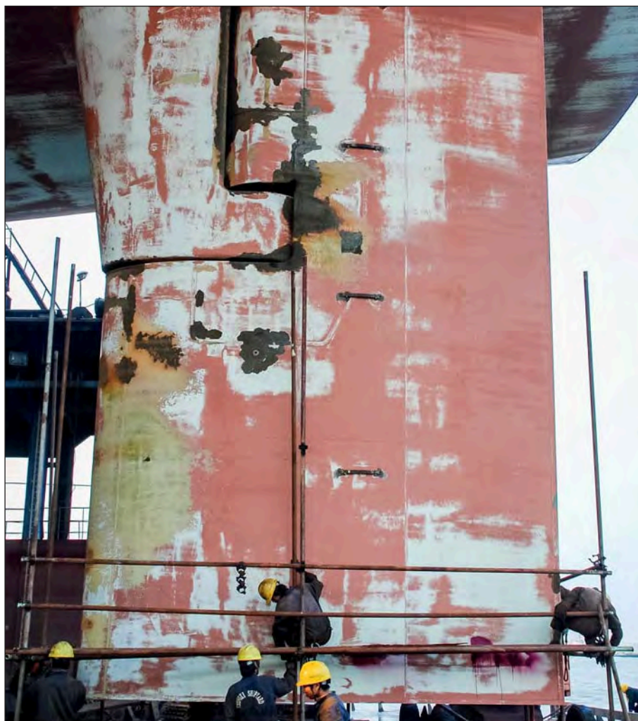
The rudder of m/v Deva when the vessel came into drydock five years ago, showing multiple damages.
