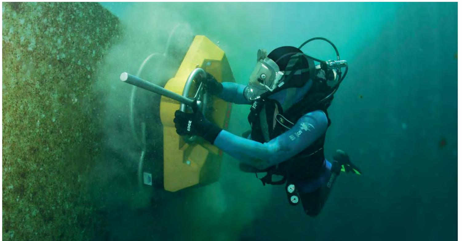
*Routine in-water cleaning keeps this cruise ship's Ecospeed coated hull clean. In fact Ecospeed gets a little smoother with each cleaning. And the cruise line is saving at least 10% on fuel costs (compared to when it was using TBT).*
