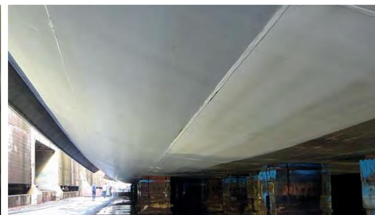
*This cruise ship came out of the water just like this. The Ecospeed coating is 5 ½ years old. It has had absolutely minimal touch-ups, no repair, no replacement. It has undergone routine in-water cleaning. The ship gained two knots over trial speeds when the coating was changed to Ecospeed. The fuel savings are enormous.*
