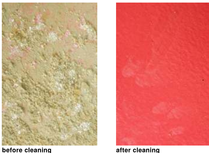
Figure 2. Before and after cleaning of a plate from Zeebrugge (1 year contact in seawater)
