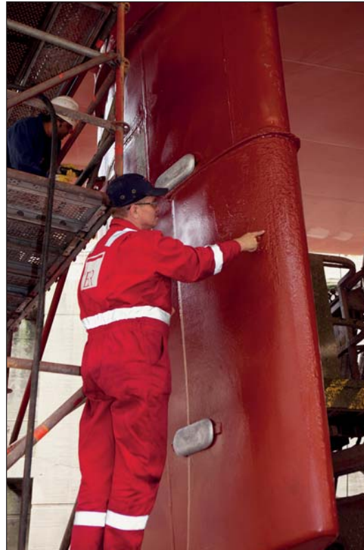
The rudder of MV Elisabeth Russ in drydock in 2011. No further cavitation damage has occurred in the intervening 7 years.
