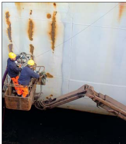
Comparative ice-strength paint on the left, Ecospeed patch on the right.
