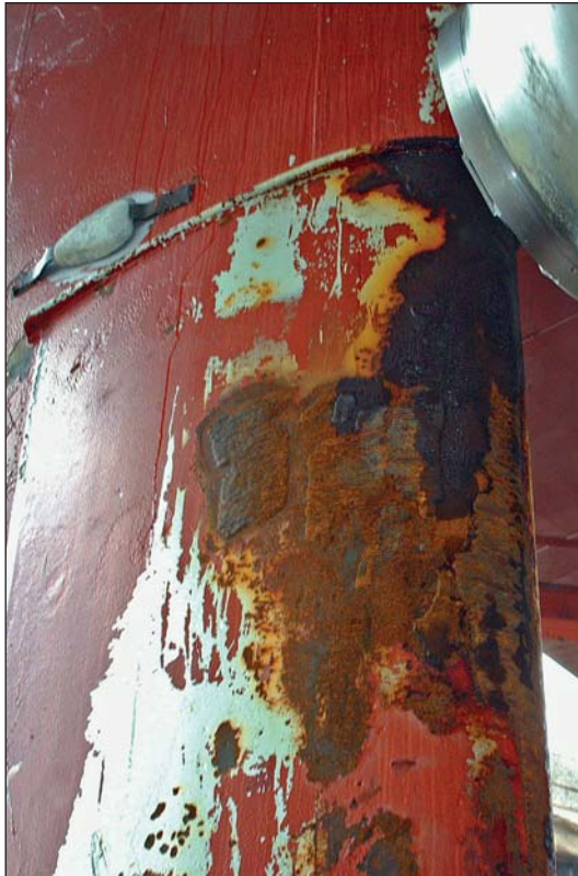
The rudder of MV Elisabeth Russ before Ecospeed was applied in 2004, showing heavy cavitation damage.
