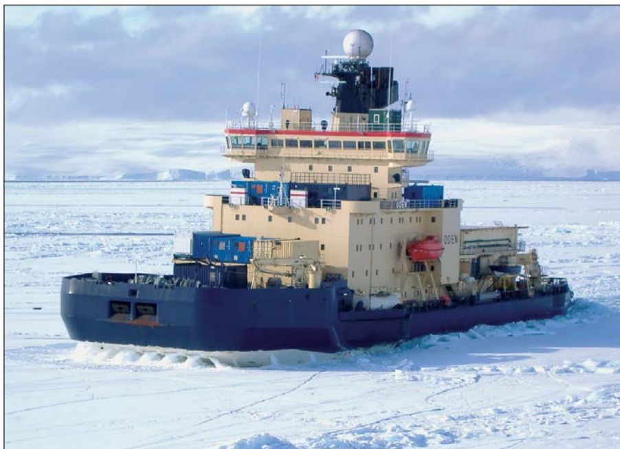
Ecospeed protects icebreaker while it crushes thick layers of polar ice
