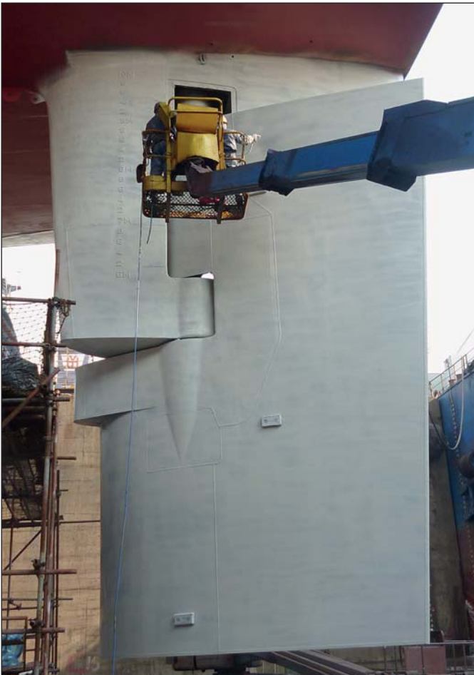
Ecoshield is applied in only two layers.
