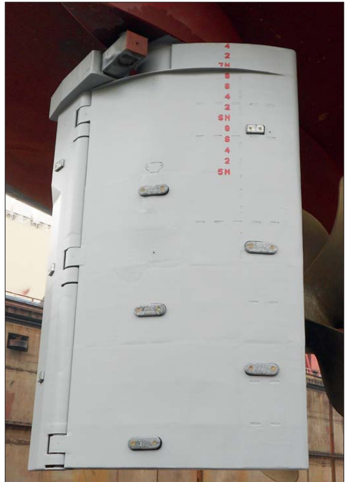
After application of Ecoshield, a rudder is protected for the rest of its service life.
