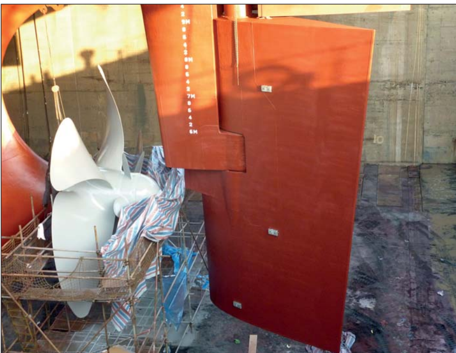
Ecoshield is the best possible protection against corrosion and cavitation damage.
