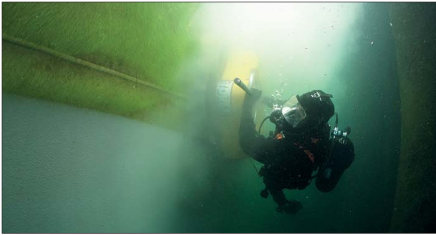
Ecospeed can be cleaned as often as needed without restrictions and without damage to the coating.
