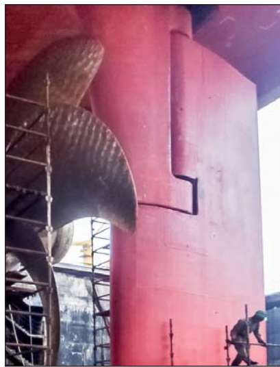
Rudder of m/v Deva after five years of service with Ecospeed.
