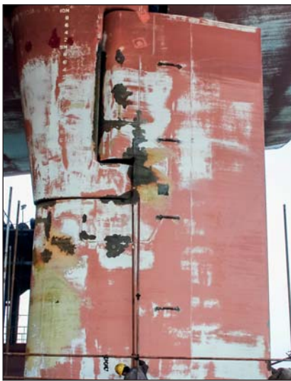
The rudder of m/v Deva when the vessel came into drydock five years ago, showing multiple damages.
