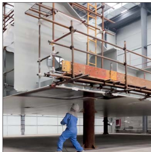
Rendering of the Caribbean FLNG (left). A hull section being coated with Ecolock (right) at Wison shipyard in Shanghai.
