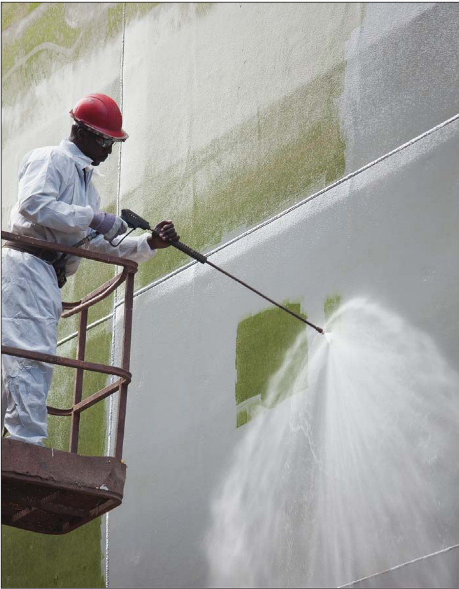
Fouling can be removed underwater or in drydock without damaging the Ecospeed coating.
