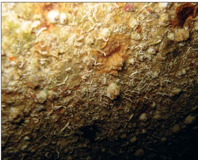
Thick layer of fouling on cruise ship after laying idle in the Caribbean for seven months.
