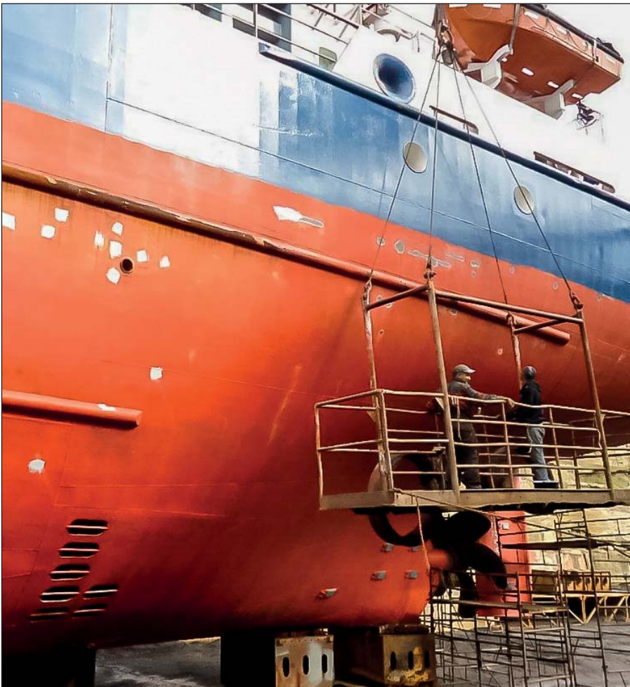
Five years after Ecospeed applied, the same hull is still smooth and the coating intact, requiring only minimal touch-ups in drydock despite trading in icy waters and no coating repair since application.
