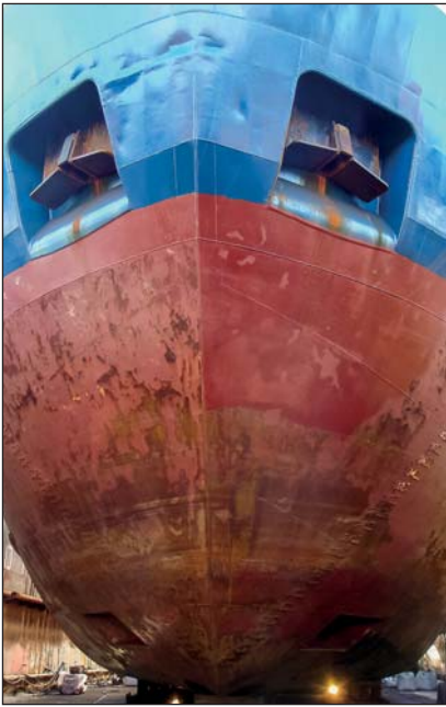
Hull of ice-going general cargo ship after a season in ice, eight years after launch with annual coating repair or replacement.
