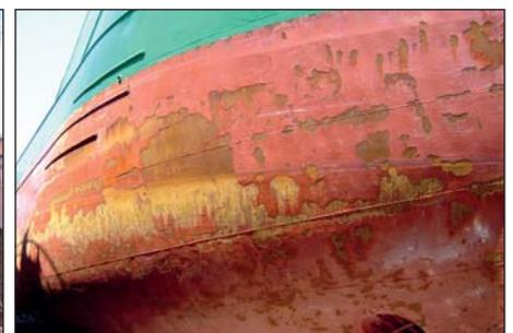
*The effect of corrosion can be devastating if the wrong protection is used for an underwater hull.*
