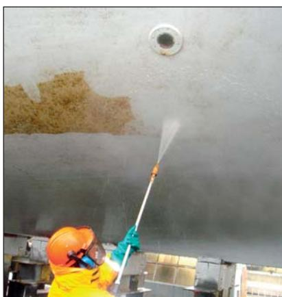
Fouling can be removed in drydock with high pressure tools or underwater while improving the coating.
