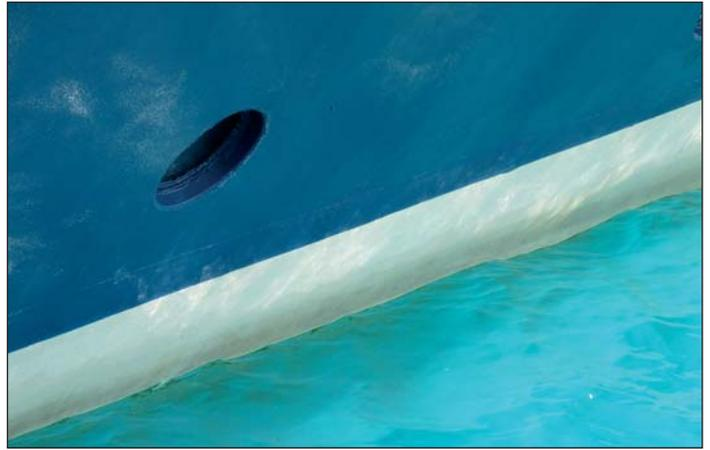
*Ecospeed coating on a cruise vessel after 6 years, seen here in drydock and in water.*
