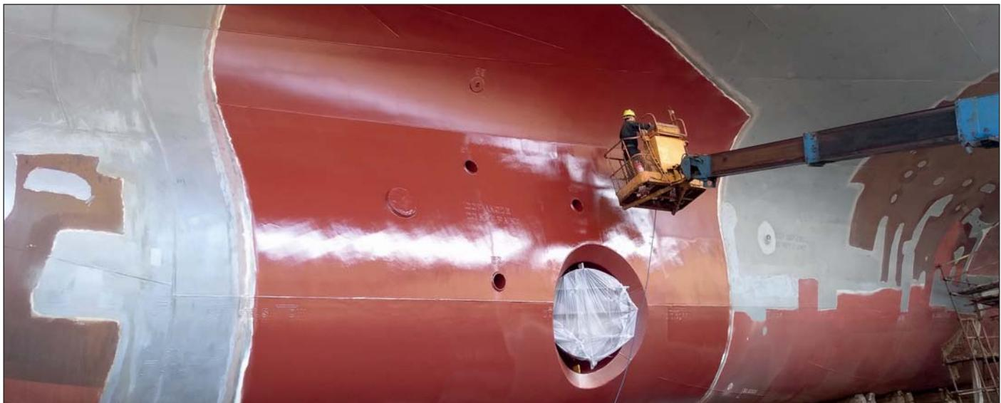
Ecospeed will protect the area around the outlets for the ship's entire lifetime.
