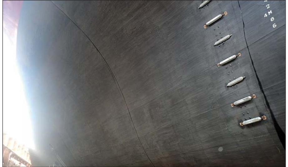
*Ship hulls coated with Ecospeed keep their sacrificial anodes intact. As a result they are no longer needed.*
