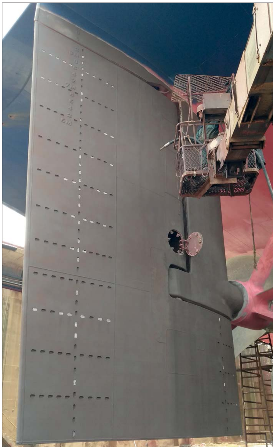
Surface preparation prior to Ecoshield application.
