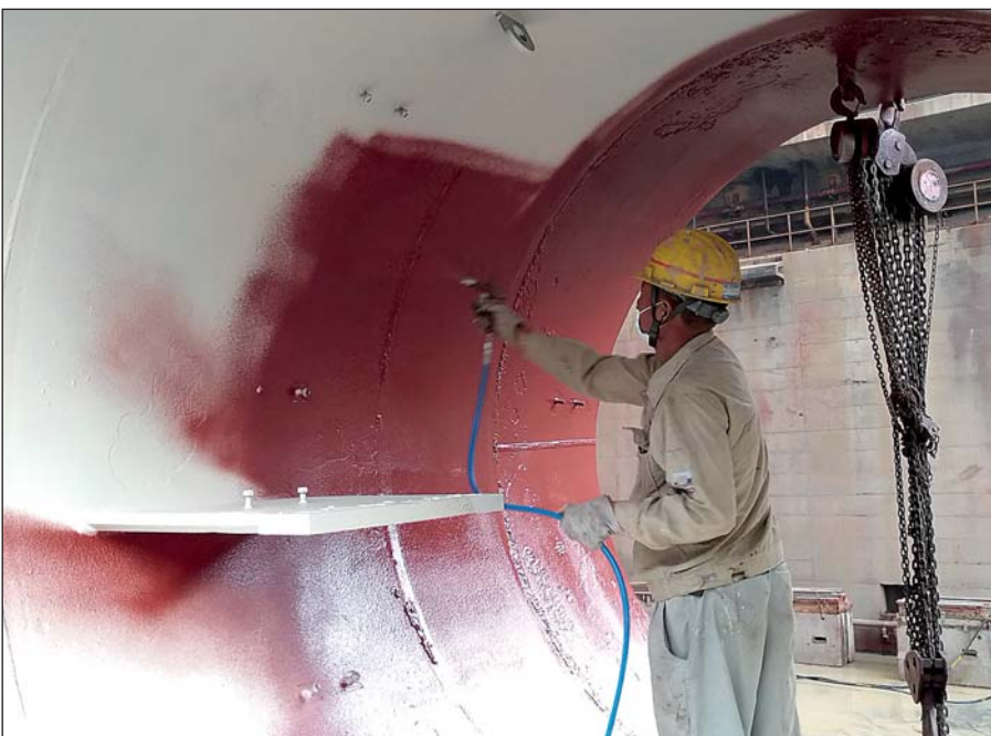
All running gear can be safeguarded from cavitation damage.
