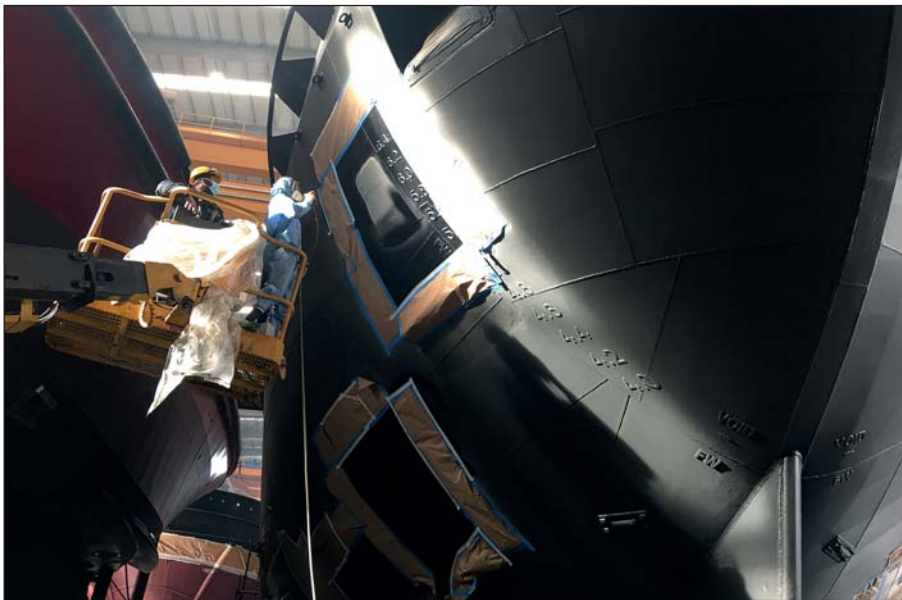
Application of the keel block areas blends in seamlessly with the rest of the coating.
