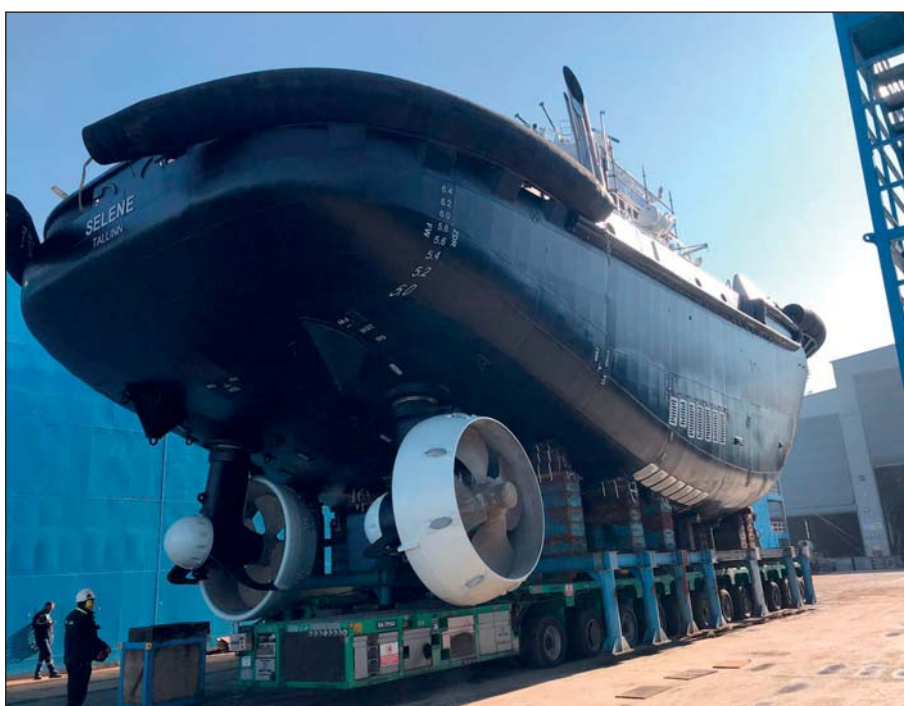
The azimuth thrusters of both vessels were coated with Ecoshield.
