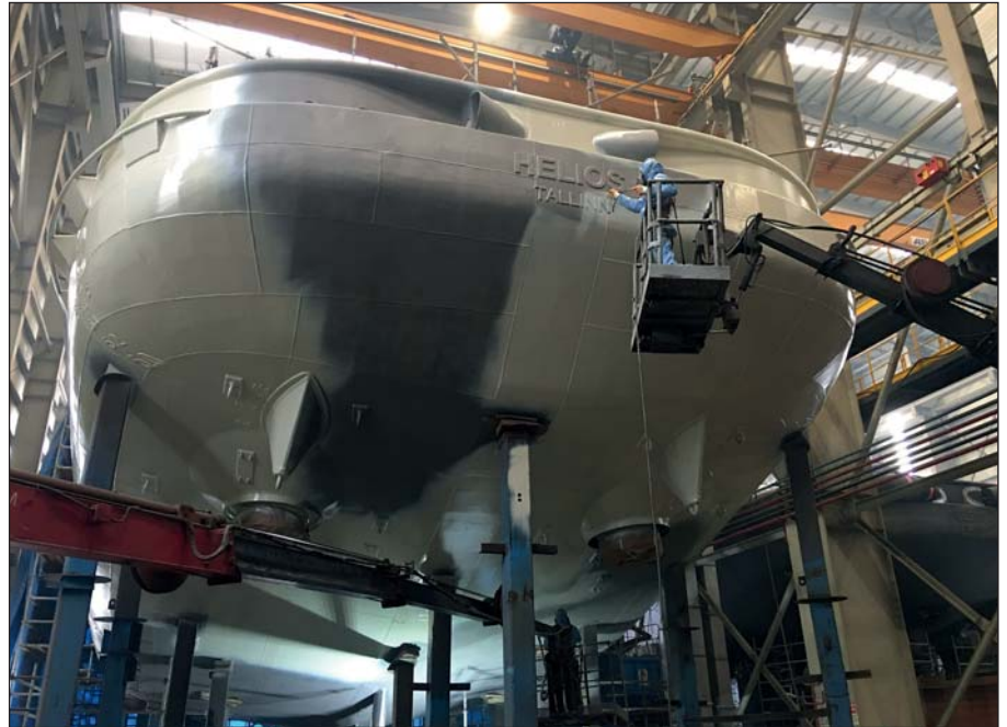
Application of first Ecospeed layer on icebreaking tug Helios.
