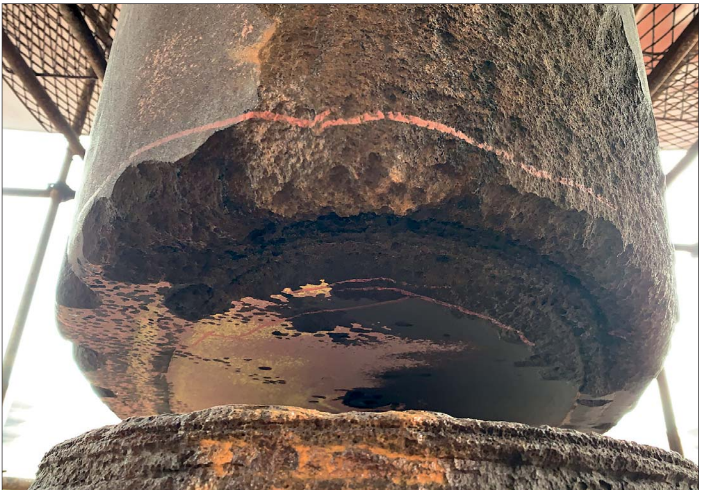
Damage like this (and much worse) occurs when running gear is not properly protected.
