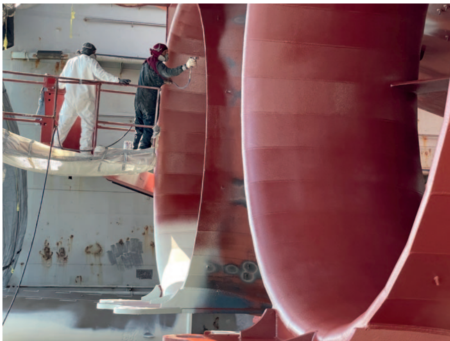
Application of second Ecoshield layer on thruster nozzle.
