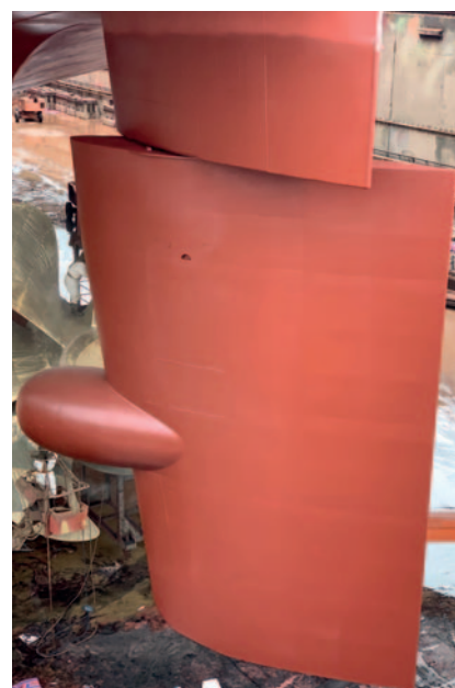
This rudder will be protected against cavitation damage for its entire lifetime.
