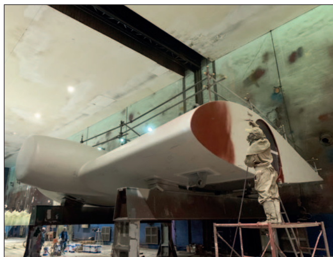
Ecoshield can be applied during the block phase or when the rudder is already attached to the ship.
