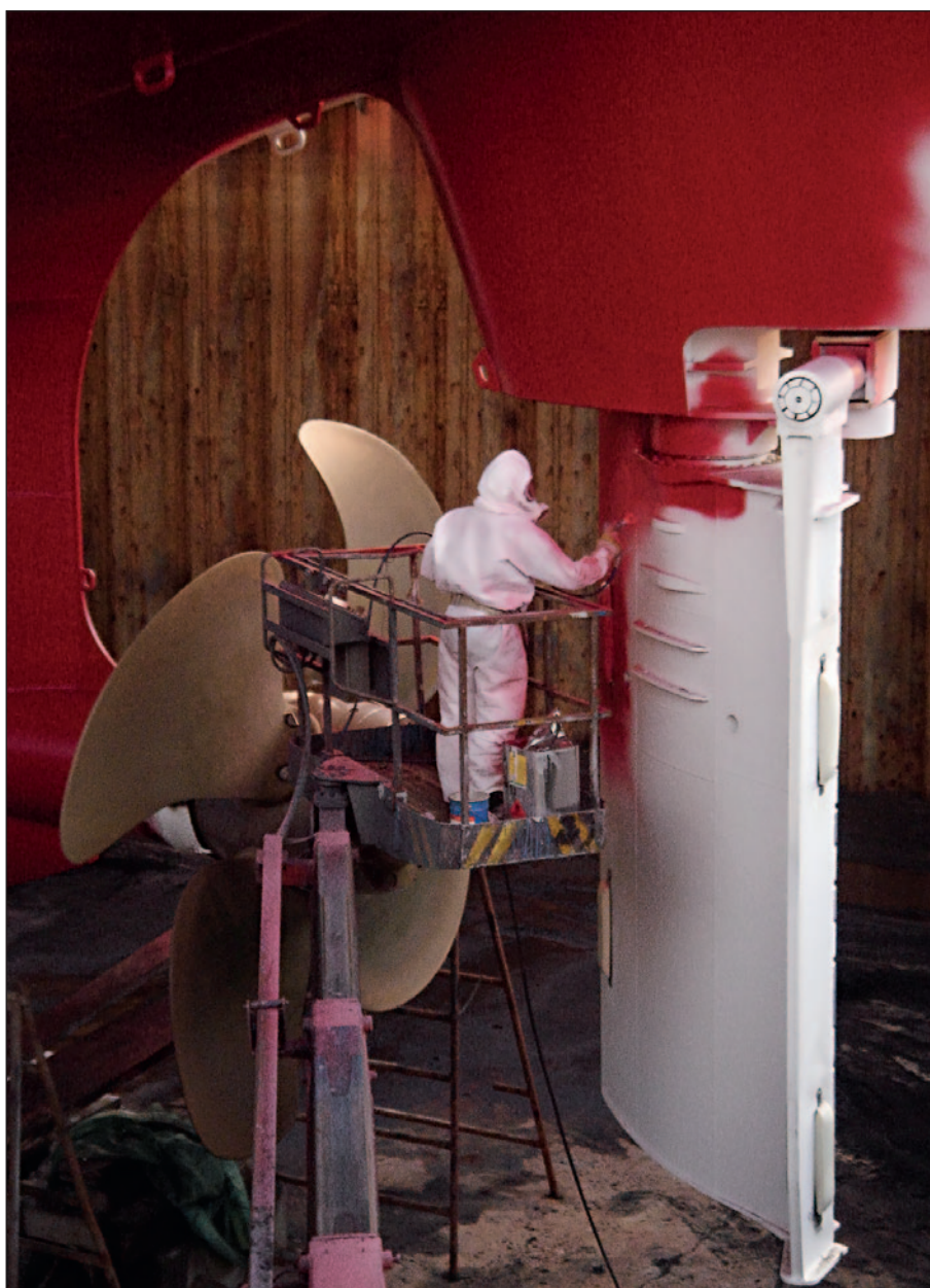
Minimum overcoat time between layers is only three hours.
