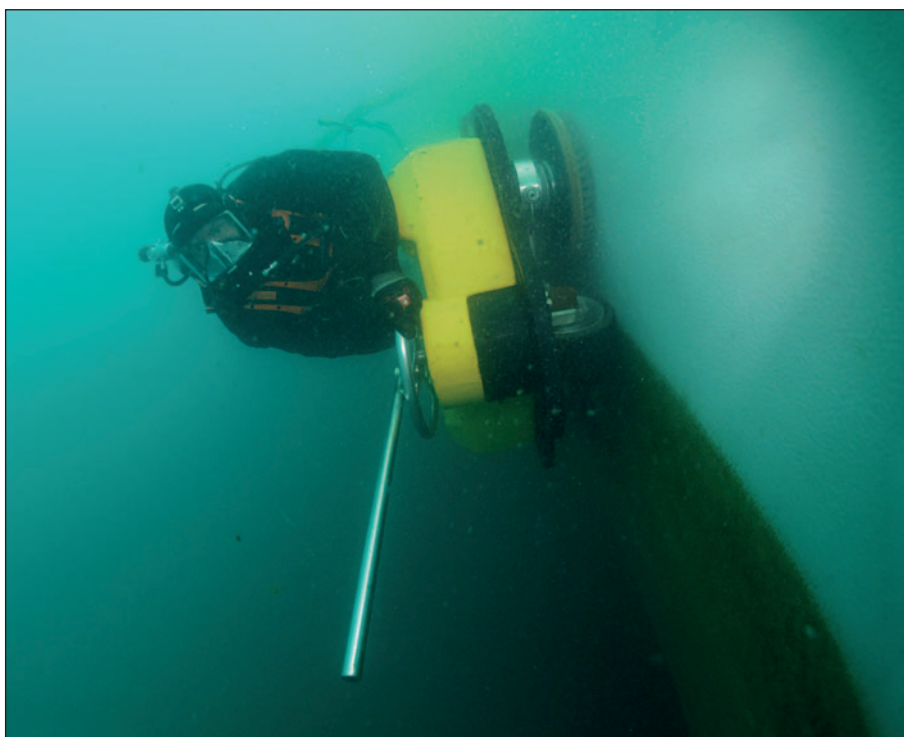
In-water cleaning of Ecospeed produces no materials that are toxic to the marine environment.
