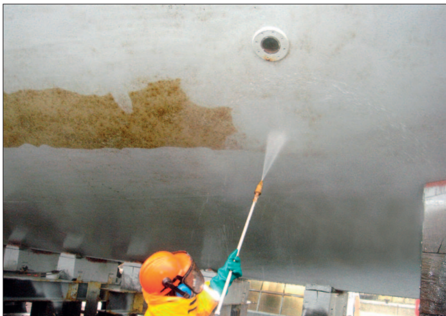
Fouling can easily be washed off in drydock with high pressure tools.
