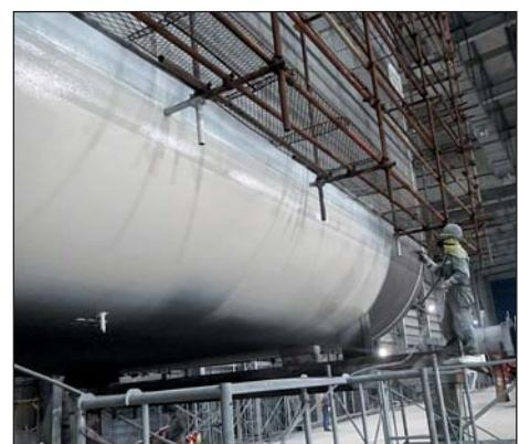
Application of Ecolock on the blocks of the FSRU.
