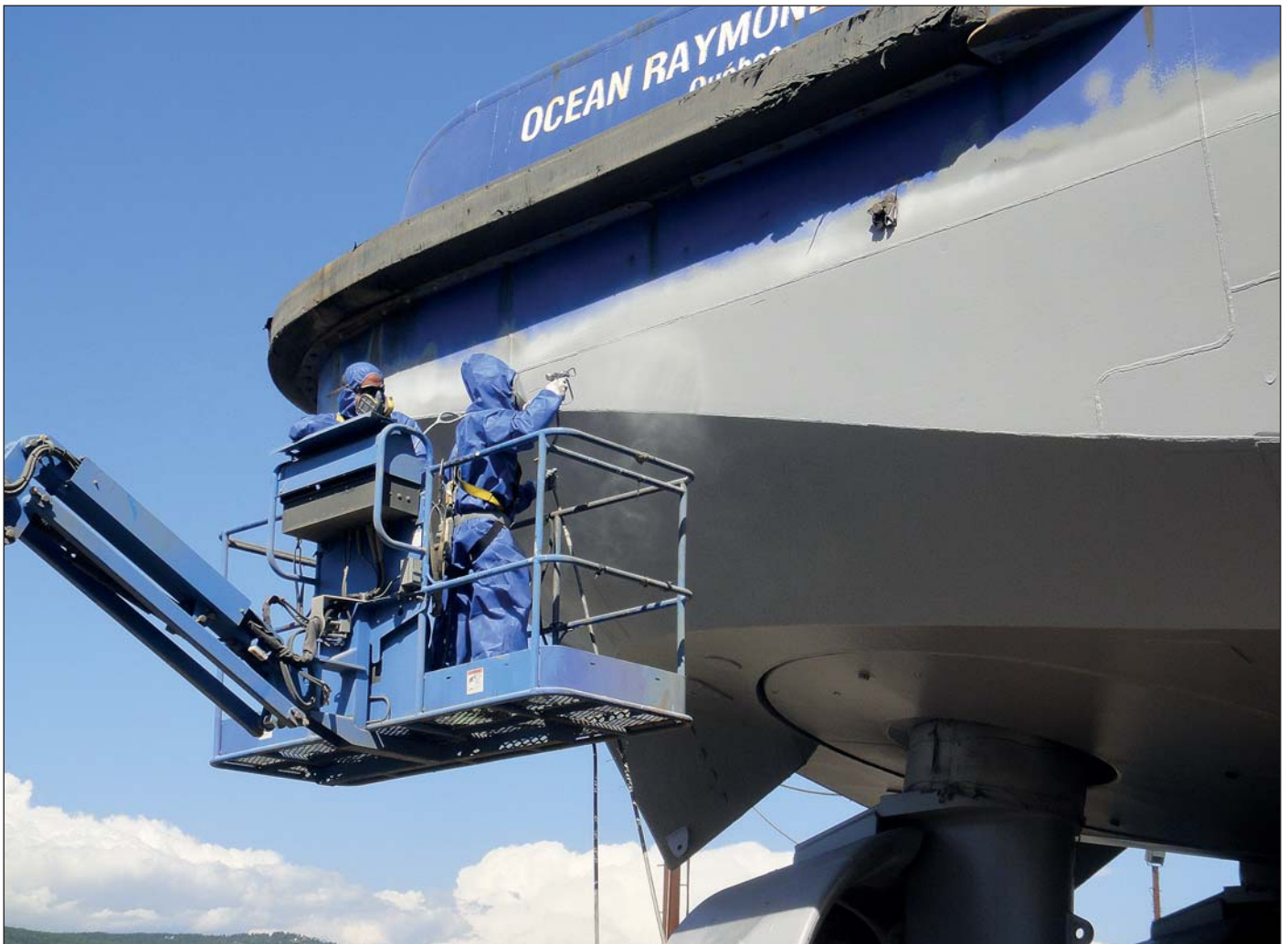
Ecospeed is expected to stay on for the life of the hull.
