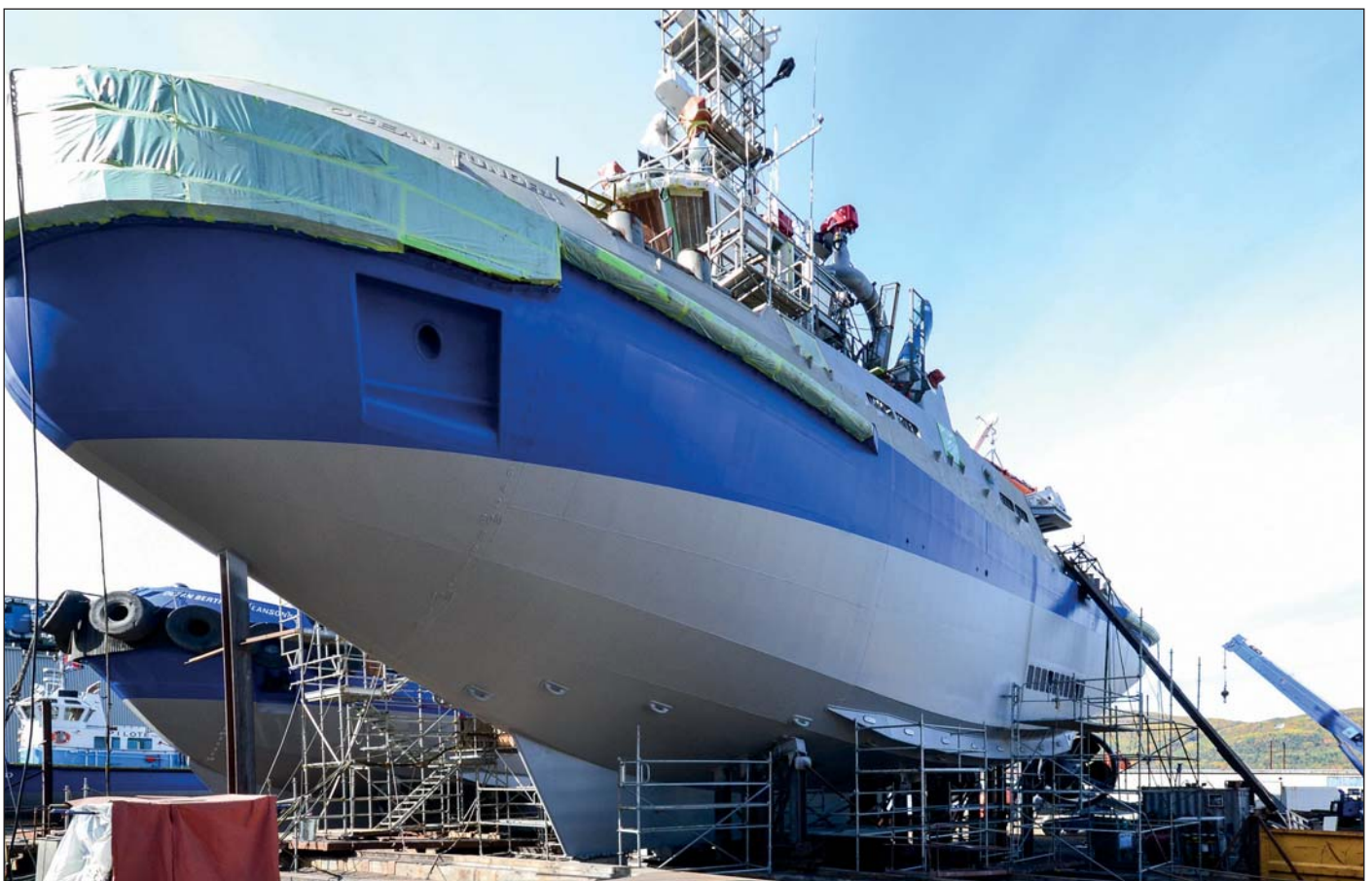
TundRA 100 with Ecospeed glassflake, ice abrasion resistant coating on hull.
