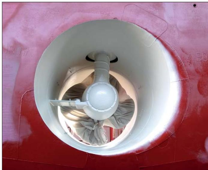
*Thruster tunnels and other running gear can also be protected with Ecoshield.*
