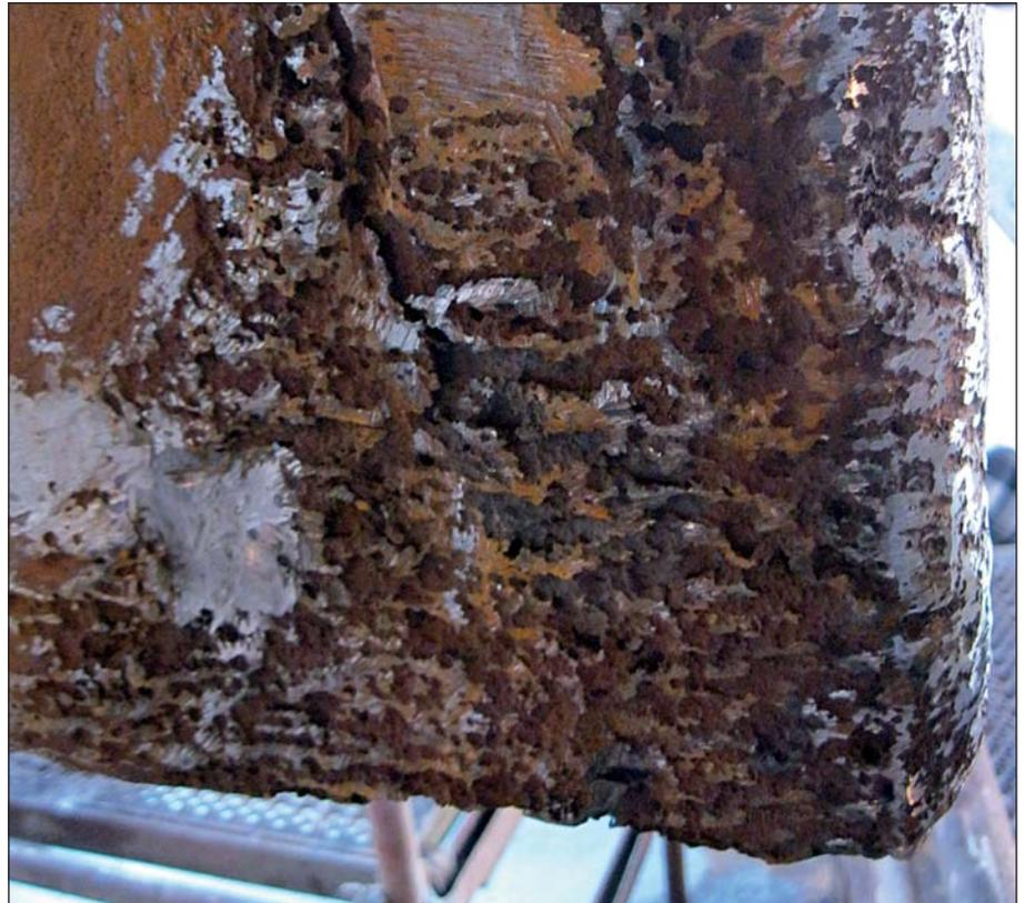
*Not protecting rudders properly can lead to very extensive cavitation damage.*
