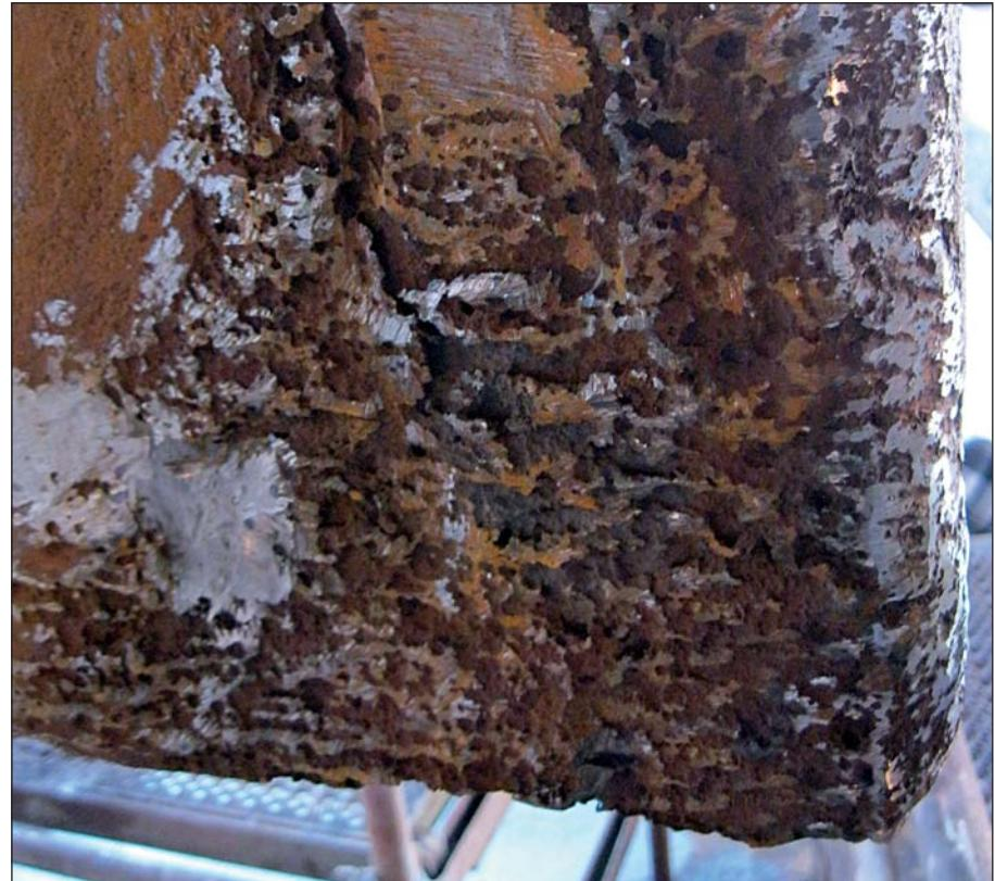
*Not protecting rudders properly can lead to very extensive cavitation damage.*
