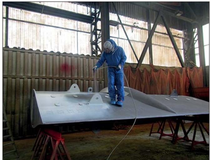
*Application of first of two identical Ecoshield layers.*
