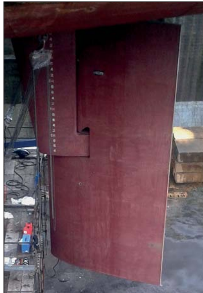
Rudder of container vessel after five years in service.
