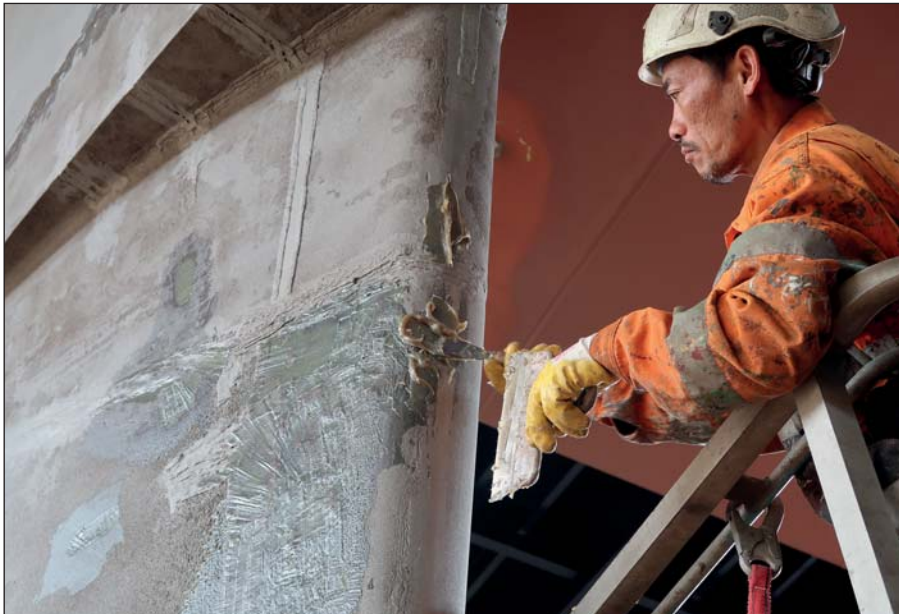
Applying Ecofix on the corroded areas of the rudder.
