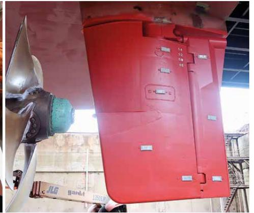
*The rudder of this roro vessel was given the full treatment in Munkebo, Denmark. First Ecofix was applied to restore the surface of the damaged rudder back to its original condition. Next it was coated with Ecoshield. This will protect the rudder from ever suffering corrosion and cavitation damage again.*
