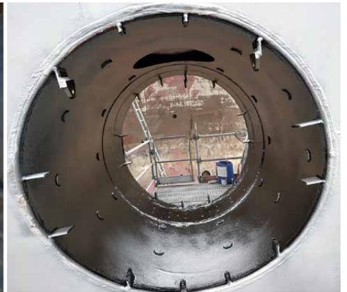
*Ecofix is also suitable for thruster tunnels and other parts of the underwater ship that need special protection from corrosion. Now these items can also be repaired prior to recoating when other, less effective coatings have permitted corrosion and cavitation damage to occur. For this reason the corrosion damage in the thruster tunnel of this container vessel was repaired in Rotterdam with Ecofix before Ecoshield was applied.*
