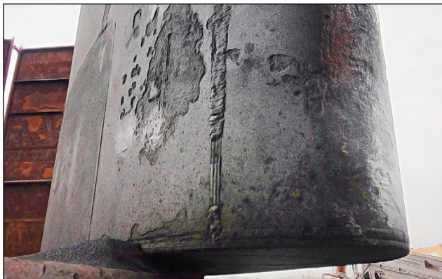
The high-powered forces of cavitation can seriously damage poorly protected rudders and running gear.
