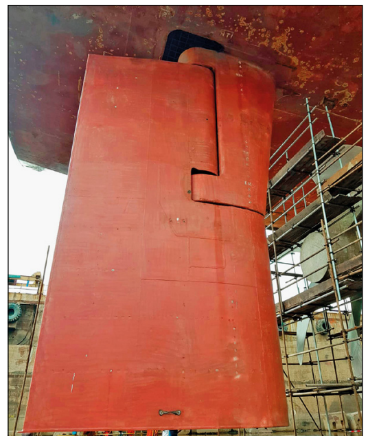
Seaspan New York 10 years after original application with no repaint.
