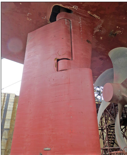
Seaspan New York (same ship) 5 years after Ecoshield application (no repaint).
