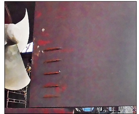
The rudder of the Pleiades vessel Xanthos. Lft. Before Ecoshield application January 2014. Ctr. Original Ecoshield application. Rt. After 7 years sailing, no repainting or repair.
