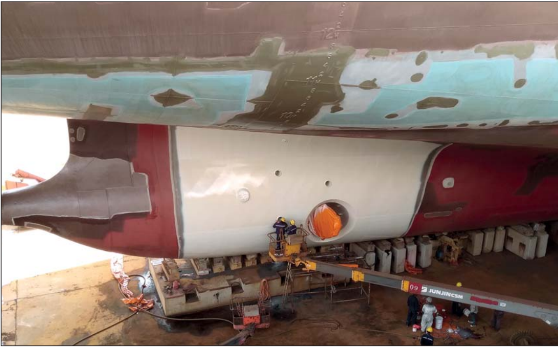
Inspection of the scrubber outlet area after application of first layer.
