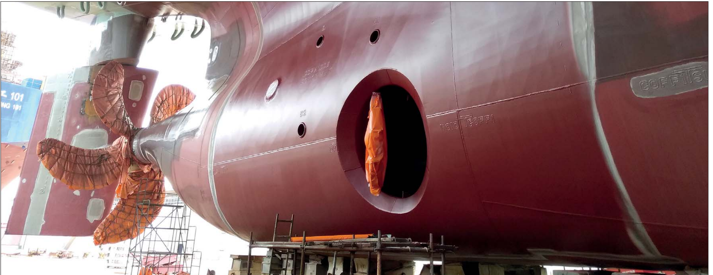
Ecospeed will protect the area around the outlets for the ship's entire lifetime.
