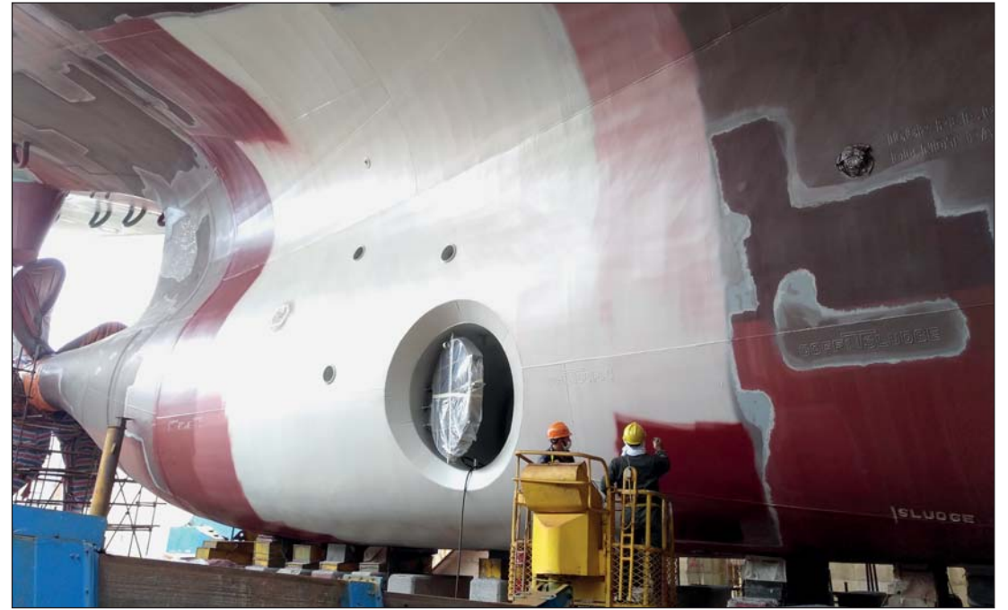
The second layer can be applied as soon as 3 hours after the first.
