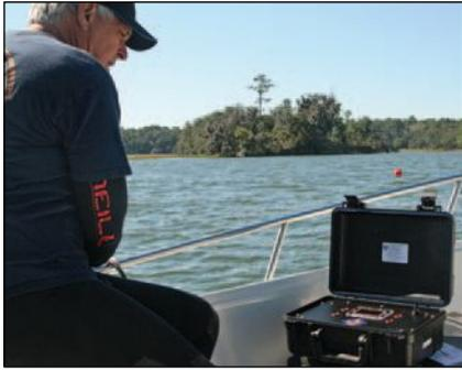
an operator range and bearing to a marked subsea target. Battery operated, the STI-350 uses a LCD to display range/signal strength and bearing to the target beacon. Sealed switches allow the operator to access the many functions of the STI-350. A rugged aluminum anodized staff assembly allows easy deployment of the highly directional hydrophone.
