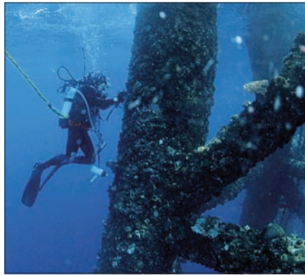
Stationary vessels are open invitations to both micro and macro fouling, especially considering that conventional biocidal antifoulants require flowing water to work
