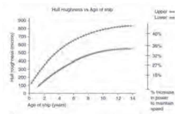
Increased average hull roughness with ship age and effect on powering with conventional coatings. Source: International Marine Coatings Akzo Nobel, Propeller Issue 15, January 2003, p 7, as used in Chapter 7 of Advances in marine antifouling coatings and technologies, edited by Claire Hellio and Diego Yebra, page 161.
