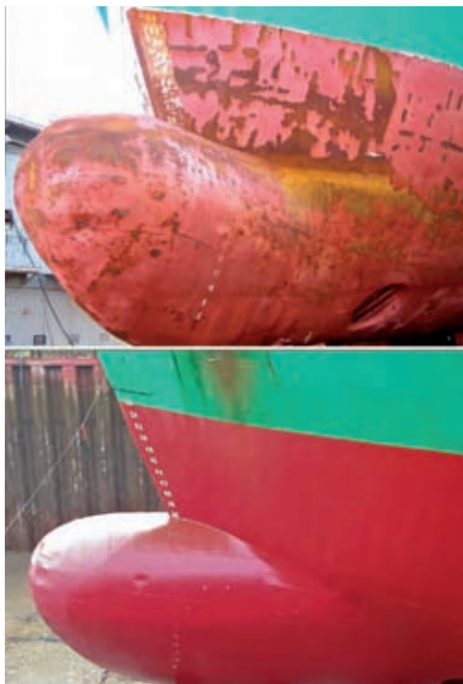
Coating comparison between conventional coating after a season in the ice (above) and a STC after two seasons in the same ice conditions (beneath).
