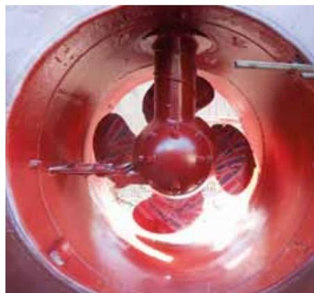
to metal facing or very expensive fillers and because it is part of the Ecospeed/Ecoshield family, it is non-toxic and extremely durable. Since Ecofix uses the same basic resin as Ecoshield, the coating can be applied just one hour after applying the filler. "Ecoshield is the only coating known to fully protect rudders and thrusters from all
