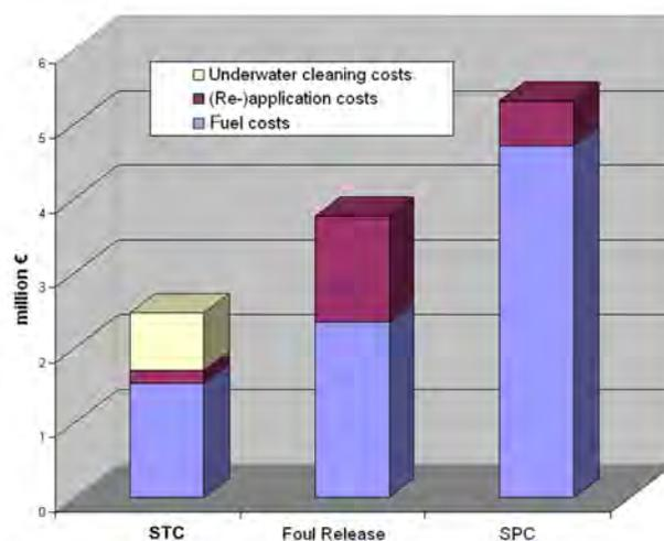
When all the costs aspects are taken together, it is estimated that the overall economical impact of [the glass flake vinyl ester STC] is less than half of that of an SPC and about  $\frac{2}{3}$  of a foul release for a 1000-TEU container vessel over 25 years.<sup>22</sup>
