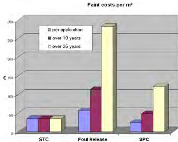
The second graph compares the total ownership cost for the three main categories of hull coating systems, including application and reapplication costs, underwater cleaning costs and the fuel costs over 25 years.
