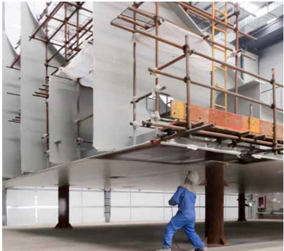
Antifouling coating during shipbuilding process
