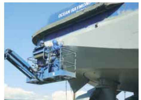
Paint crew applying top coat of Ecospeed
