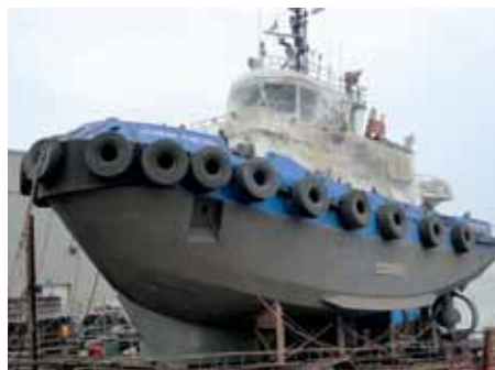
Hull of Ocean Raymond Lemay blasted ready for painting
