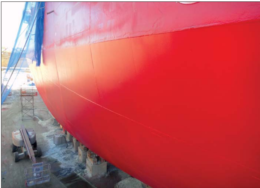
After Ecospeed application the hull of the vessel is protected against even the harsh icy condition of the Antarctic region.
