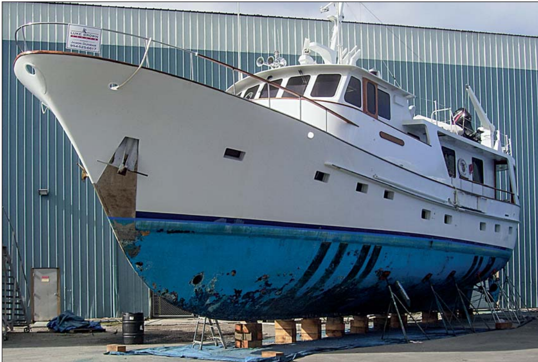
The Oceantide out of the water just before the hull was grit blasted and Ecospeed was applied.
