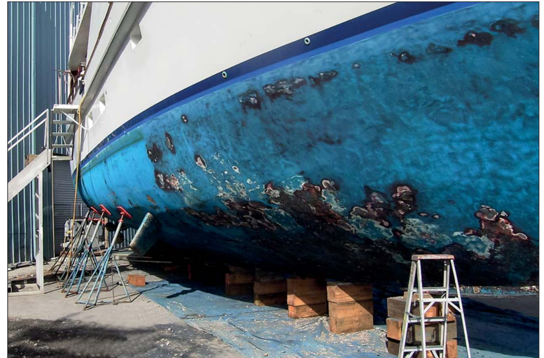
Detail of the condition of the hull in 2007 prior to Ecospeed application.
