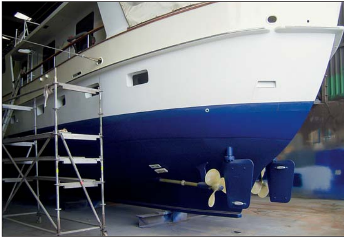
Newly applied Ecospeed on the hull.
