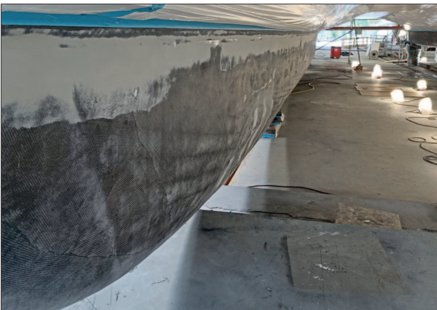
The hull of the energy-efficient sightseeing catamaran is made of carbon fiber.
