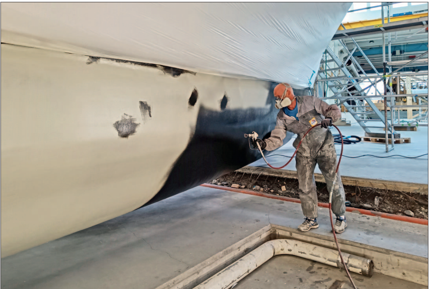
Overcoating time between layers is very short. Smaller projects like this can be completed in a single day.
