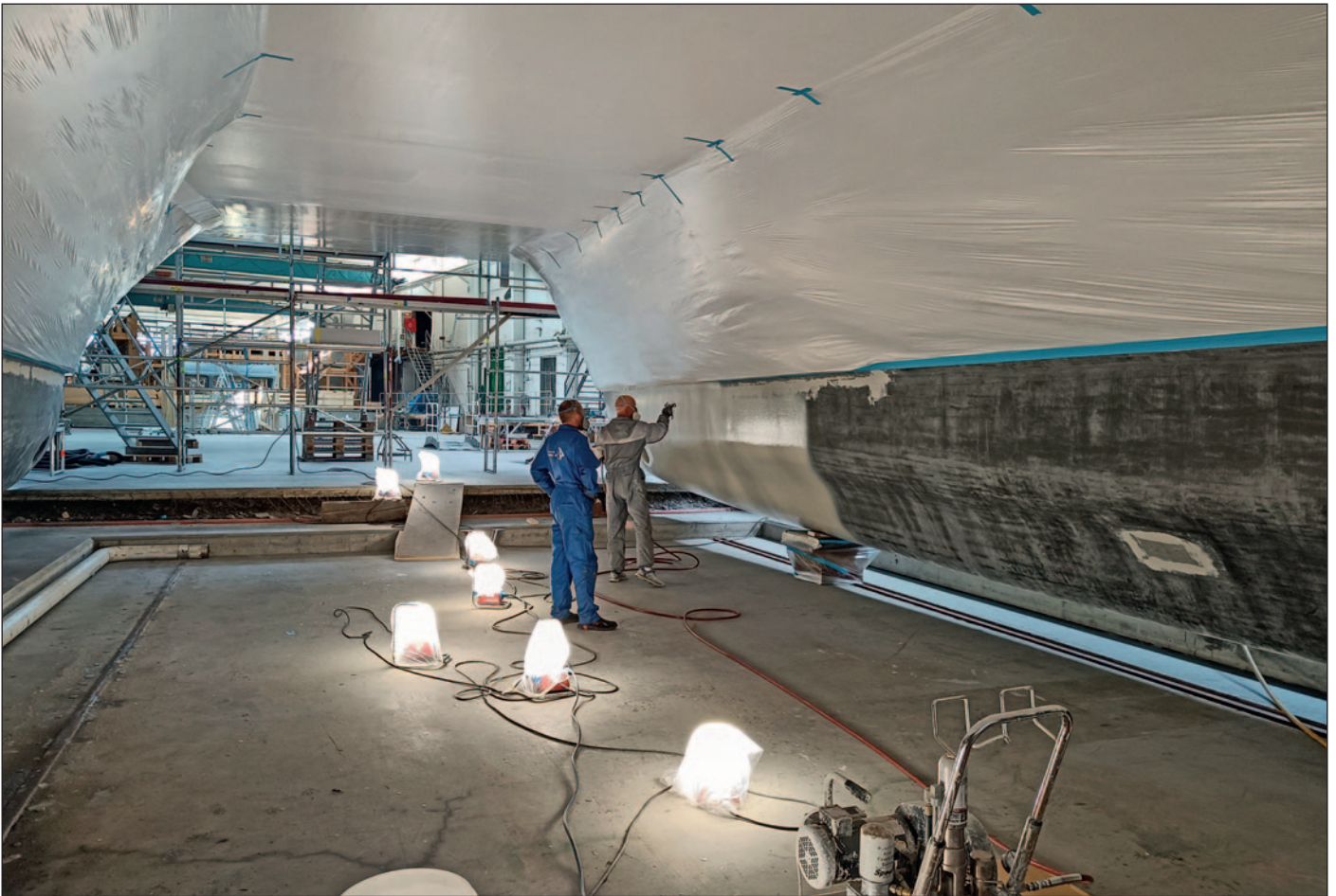
Ecospeed is applied in two layers and offers a lasting non-toxic protection.
