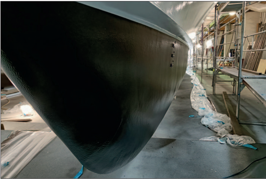
No repaint will be needed during future dockings, only small touch-ups.
