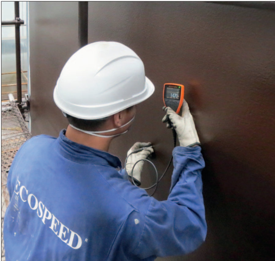
Raul Yu inspecting the final coating on the EXMAR LNG newbuild at Wison shipyard as part of Carich's work with Subsea Industries to deliver Ecolock.
