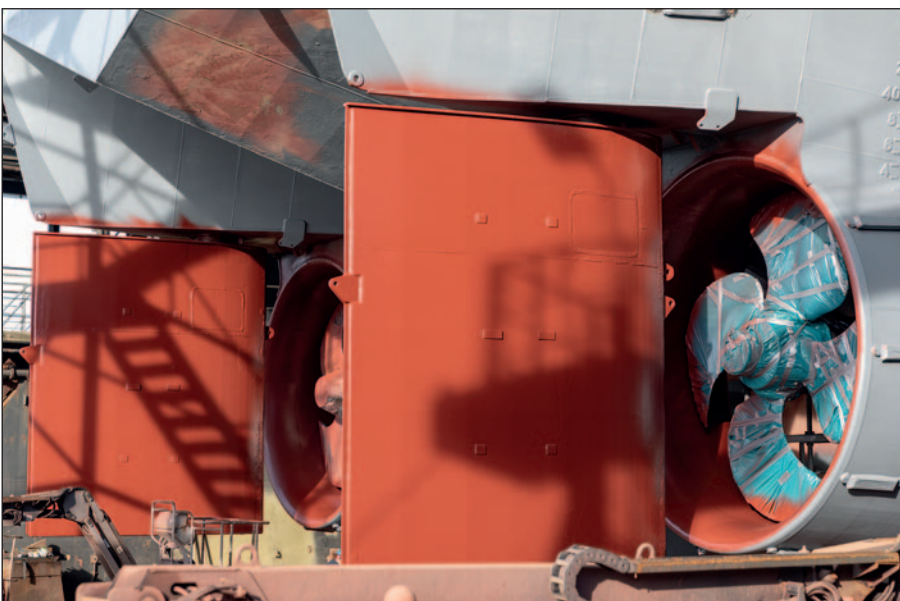
Double rudders on dredger, both have been coated with Ecoshield.
