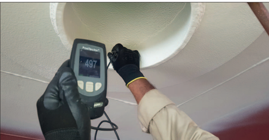
Ecospeed surveyor inspecting the layer thickness.
