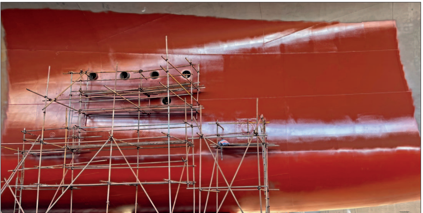
The second layer can be applied as soon as 3 hours after the first.
