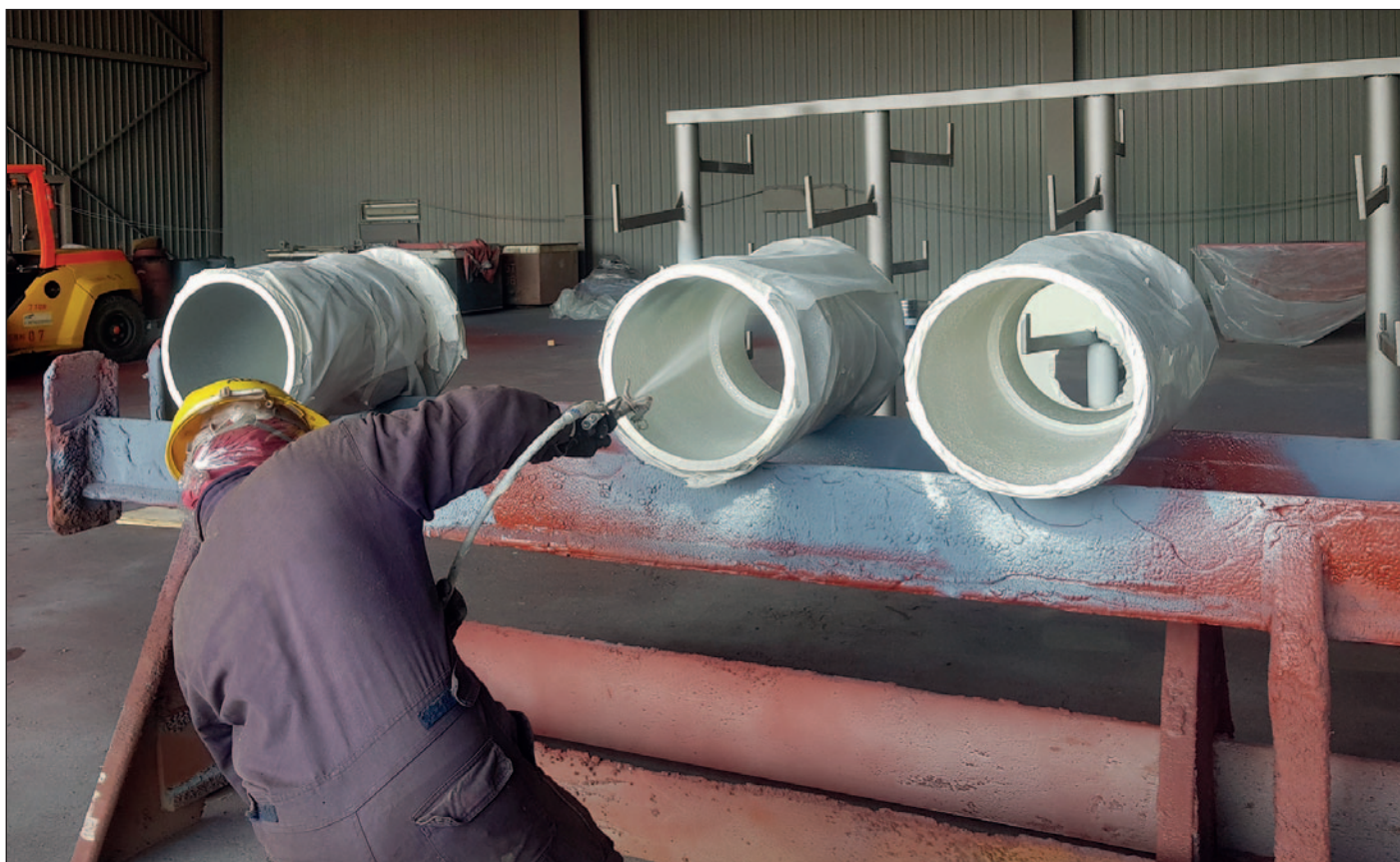
Application of first Ecospeed layer on scrubber pipes.
