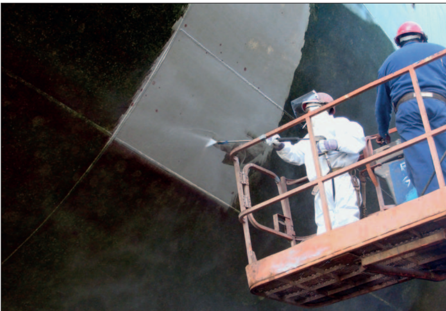
With Ecospeed the coating is always in an as new, excellent condition after a high pressure washing.
