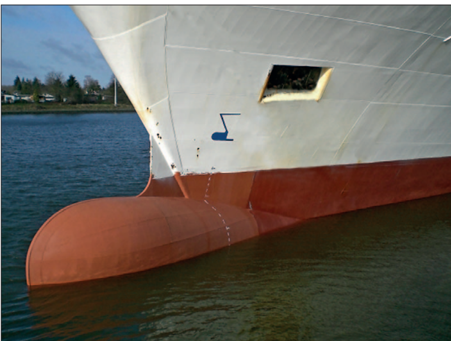
The bulbous bow of the Friedrich Russ one year after it was coated with Ecoshield's predecessor Ecospeed, including a winter sailing in ice.
