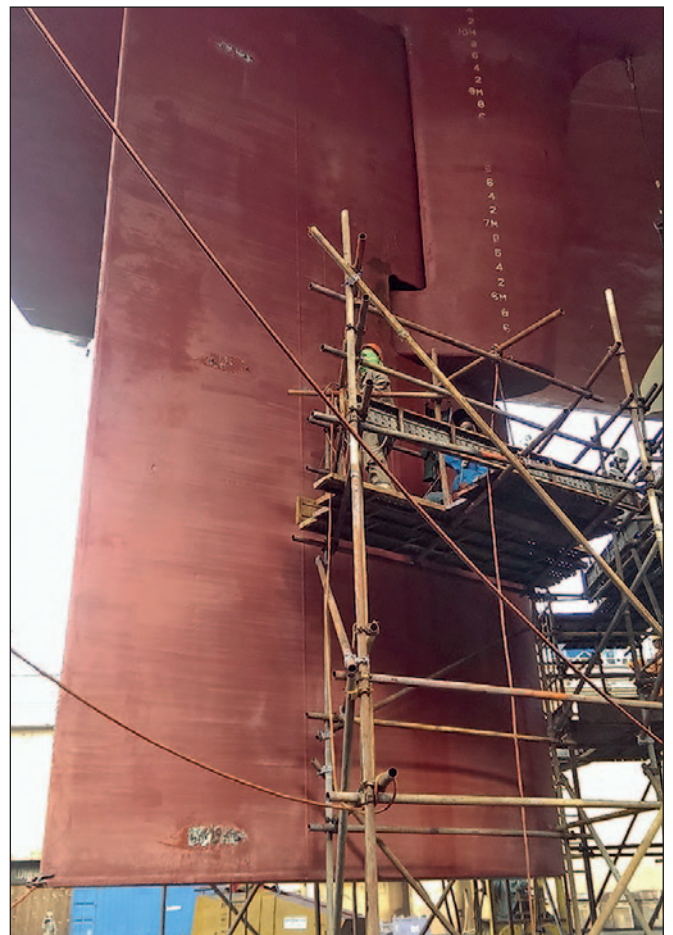
Rudder of the Seaspans Santos 8 years after Ecoshield was applied, with no repaint during that time.
