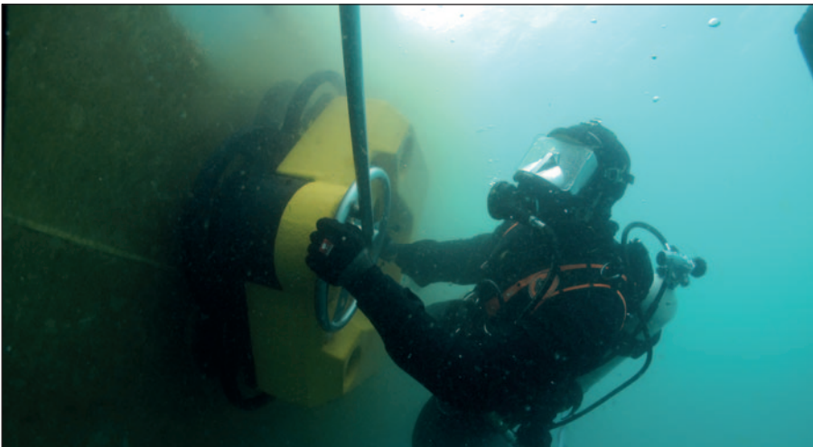
Ecospeed underwater maintenance is carried out with specially designed equipment.
