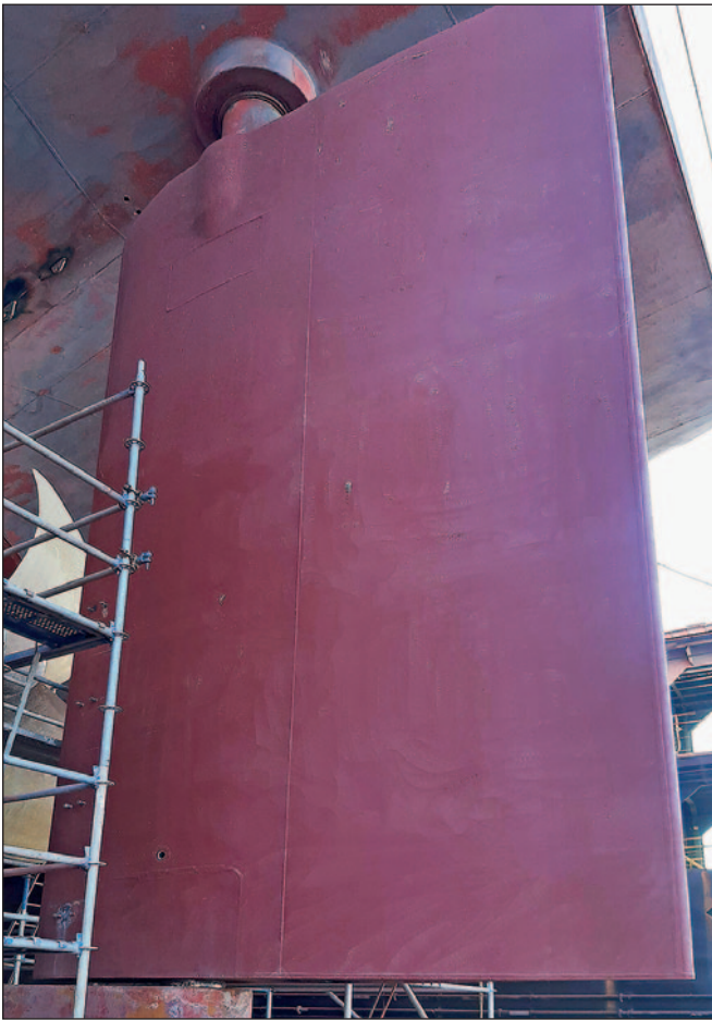
The rudder of the Pleiades Evrotas after being washed down in drydock, 5 years after initial Ecoshield application (no repaint).
