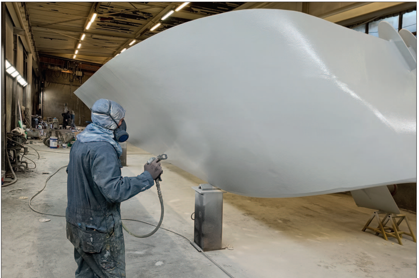
Ecoshield being applied to a Hull Vane for a navy ship.
