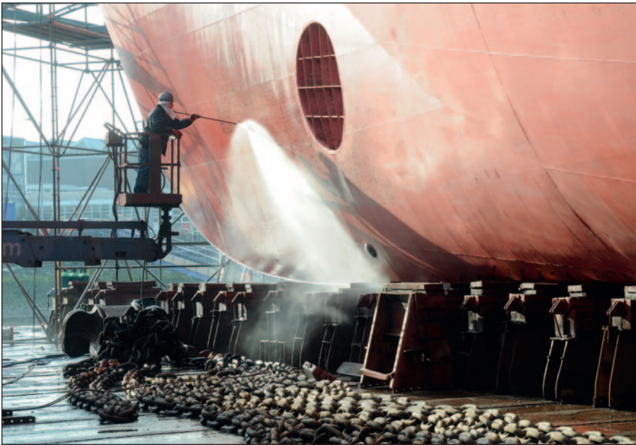
Fouling can be washed off in drydock with high pressure tools or underwater while improving the coating.
