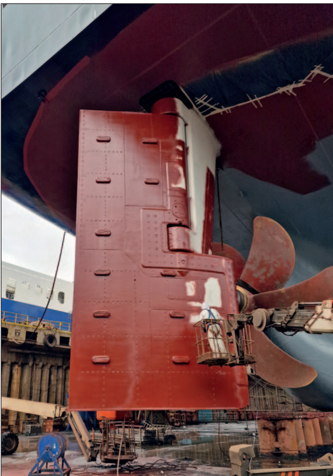
Rudder of the MSC Ziata R with second coat of Ecoshield almost complete.
