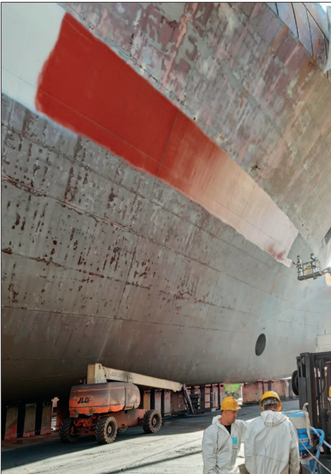
Applying the second coat (red) of Ecoshield to the boot-top of the MSC Vanquish II.
