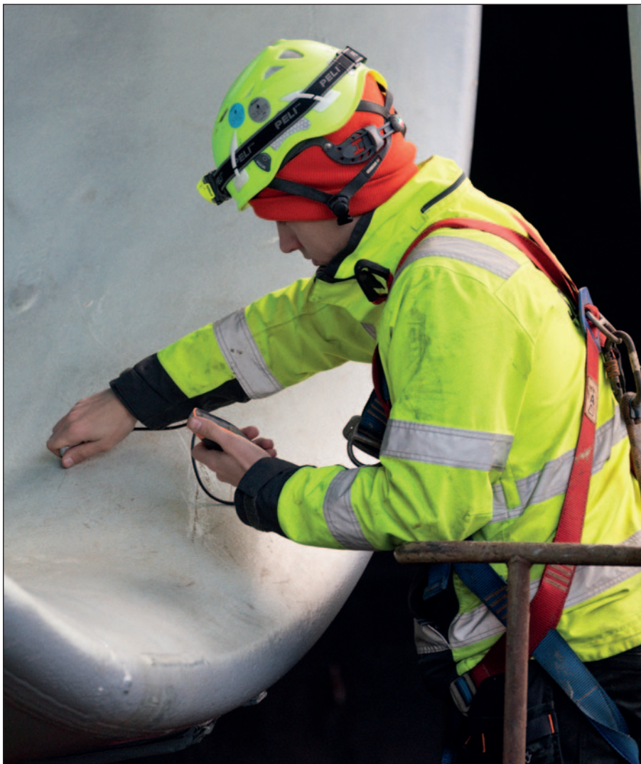
SCICON worldwide paint inspector verifying the preparation of a Kort nozzle for DEME dredger Charlemagne.
