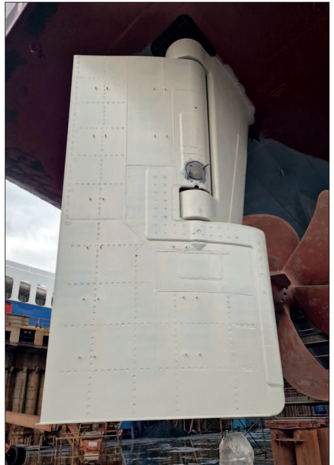
Rudder of the MSC Ziata R after the first coat of Ecoshield has been applied.
