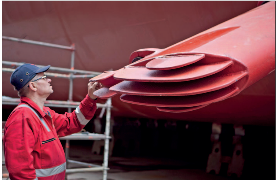
Grzegorz Girjat, Superintendent at Ernst Russ, inspecting the Ecospeed coated stabilizer fin of the Elizabeth Russ.
