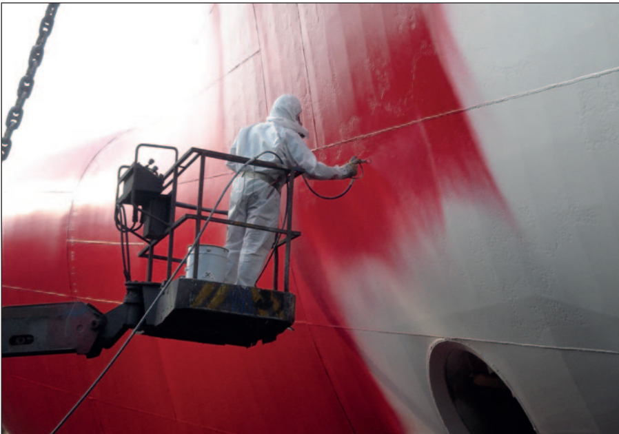
Ecospeed is applied in only two, homogeneous layers.
