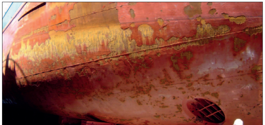
The effect of corrosion can be devastating if the wrong protection is used for an underwater hull.
