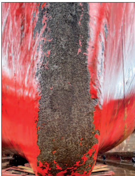
One of the test patches applied to the bow area of the Umiak I shown here 5 years after application in excellent shape compared to the existing hull coating.
