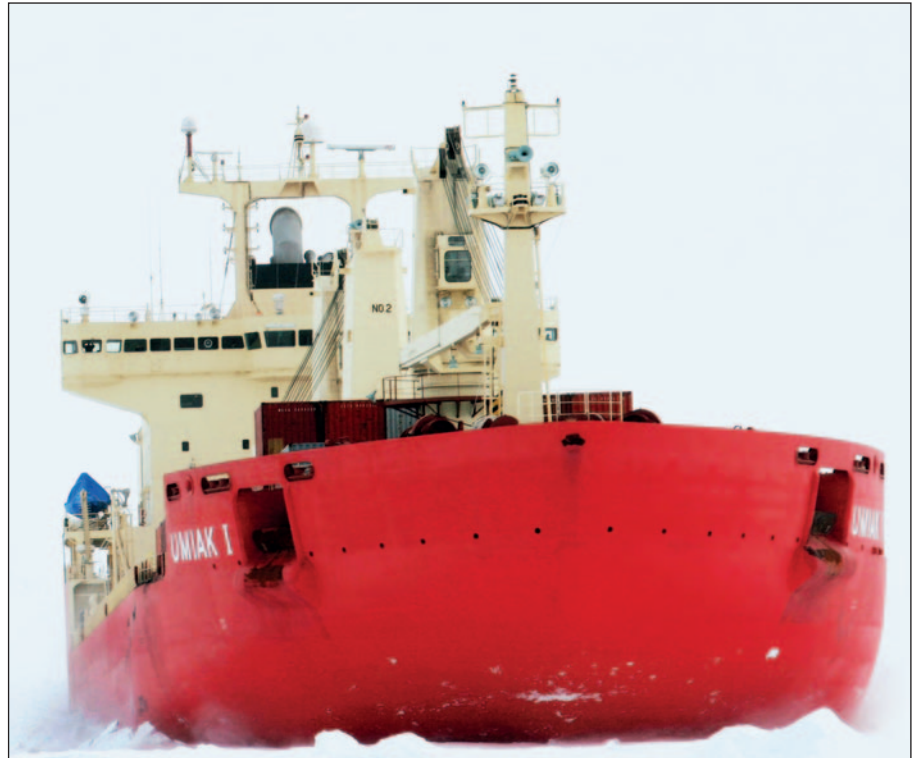
Fednav's Umiak I, DNV ice-class ICE-15, one of the most powerful icebreaking cargo ships in the world.
