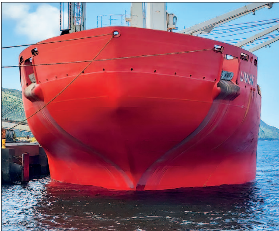
The Umiak I moored at Long Harbour, N.L. in July 2023, more than two years after Ecospeed Ice was applied to the hull.
