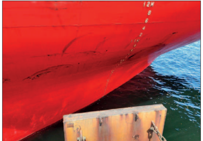
Photos of the Umiak I at Long Harbour in July 2023 showing the condition of the Ecospeed Ice hull coating after two years of plowing through heavy ice. (Photos courtesy Craig Verge, Ship Superintendent.)
