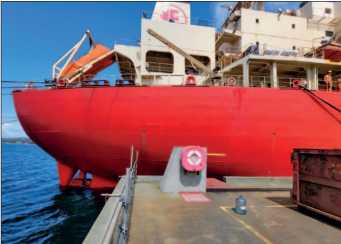
Photos of the Umiak I at Long Harbour in July 2023 showing the condition of the Ecospeed Ice hull coating after two years of plowing through heavy ice. (Photos courtesy Craig Verge, Ship Superintendent.)
