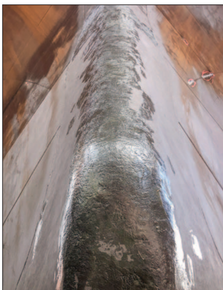
Ecofix used to repair severe pitting prior to application of Ecospeed
