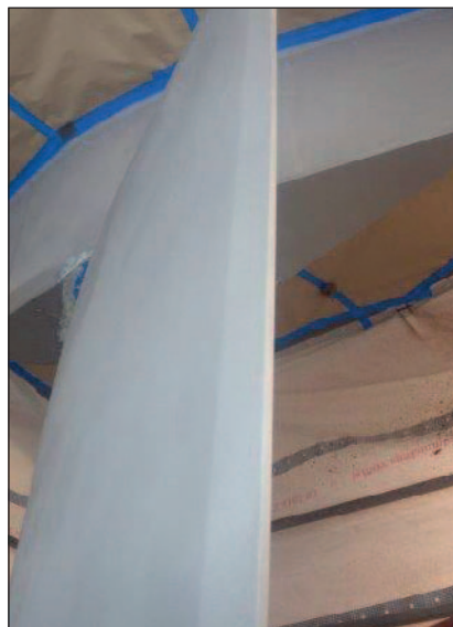
Rudder grit blasted to 2.5 SA cleanliness and a profile of 75µm ready for Ecoshield first coat.
