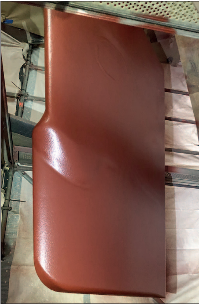
Finished rudder coated with two coats of Ecoshield for protection against cavitation.
