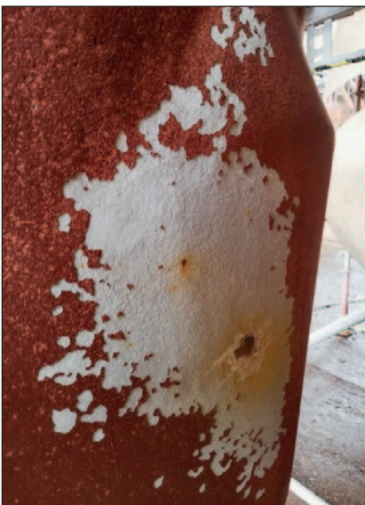
The rudder of one of the SA'AR 6 corvettes after a few days of sea trials with conventional hull coating on the rudder.
