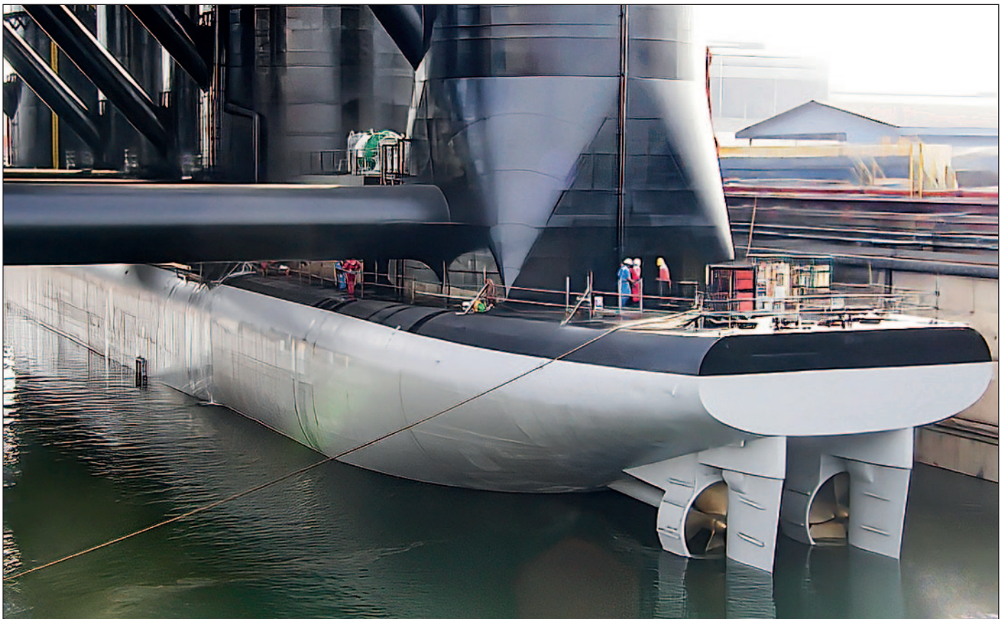
Semisubmersible coated with Ecolock. Lifetime protection, no cathodic protection.
