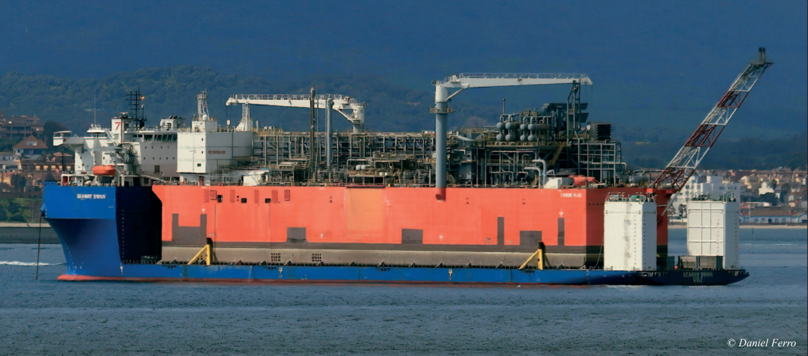
Same LNG barge 9 years after hull coated with Ecolock. No repaint. No cathodic protection. Coating intact.
