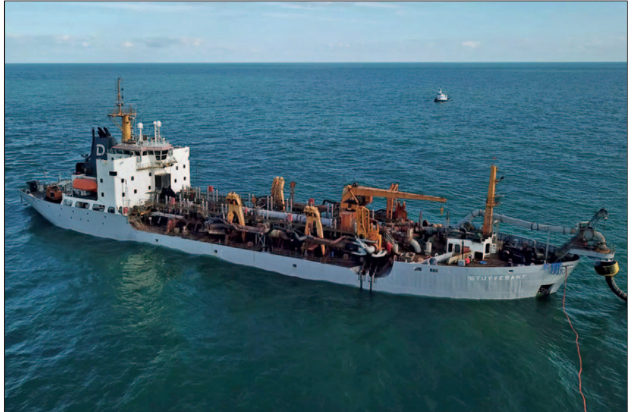
The Trailing Suction Hopper Dredger Stuyvesant is an important element of Dutra Group's fleet.
