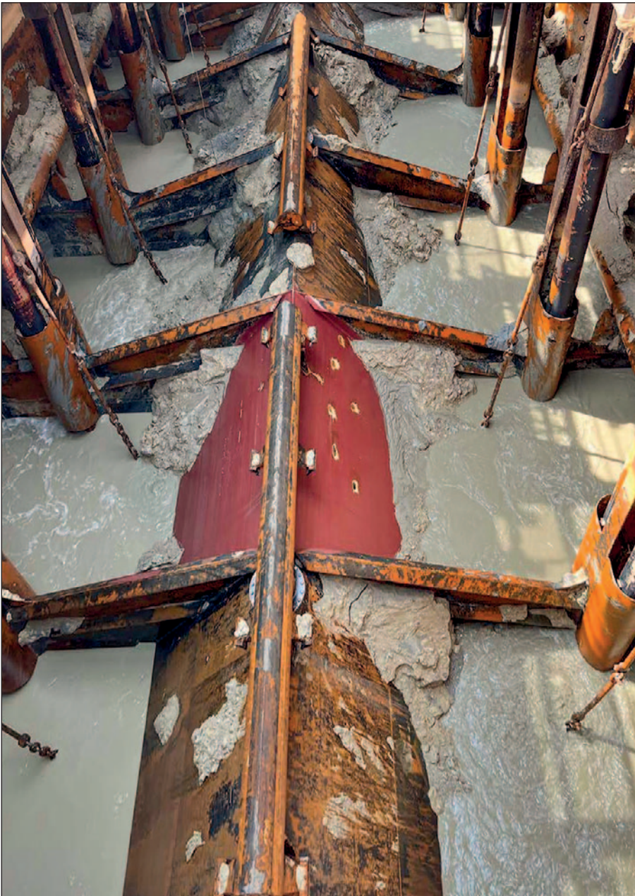
The hopper Ecoshield test patch after 10 months of active duty is in excellent condition.
