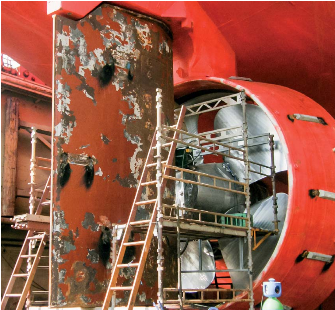
Rudder of ice-breaker/supply/research ship after a season in ice with conventional specialized ice abrasion resistant coating (the hull has Ecospeed).
