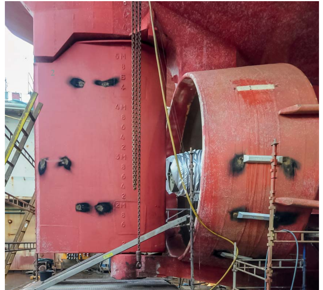
Same rudder after 2 seasons in ice after Ecoshield applied. Very minor touch-ups required. The main hull has had Ecospeed for 4 seasons.
