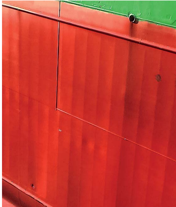
Same ship, same conditions, two years after Ecospeed applied, no repaint.
