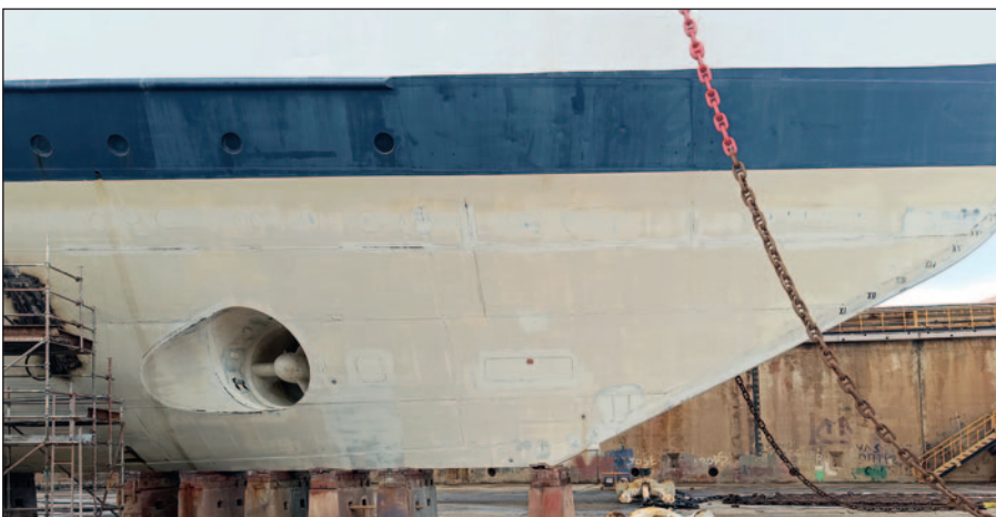
Ecospeed still intact 15 years after application on cruise vessel. This proves that the coating allows shipowners to keep the waterline of their vessel in pristine condition.
