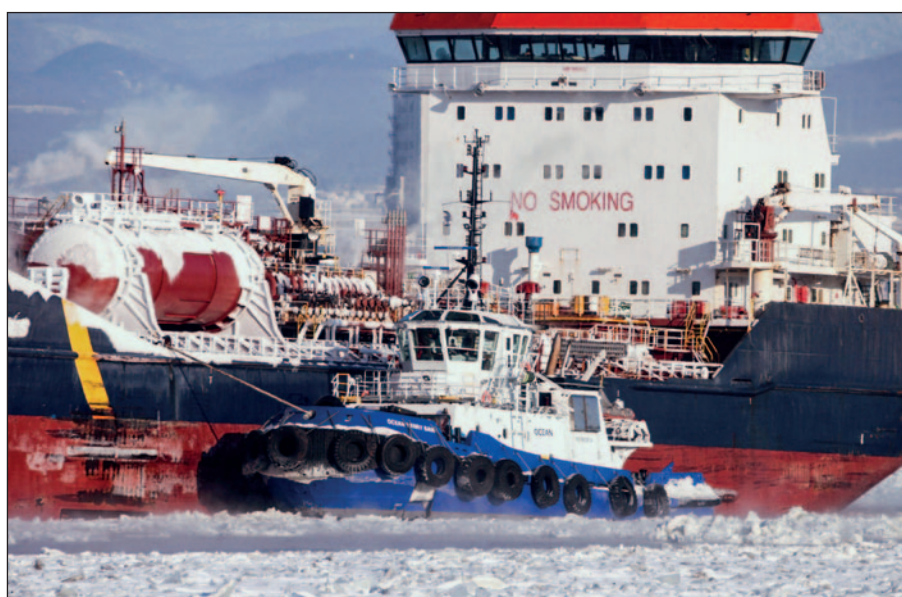
Ocean Henry Bain tug with Ecospeed Ice on the hull for full protection against the very harsh conditions of the St. Lawrence river and the Great Lakes.
