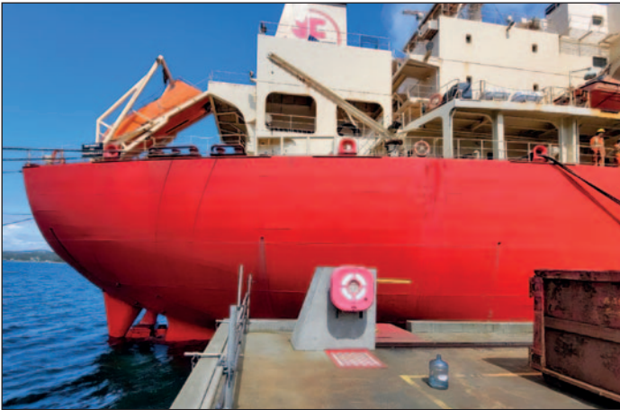
Photos of the Umiak I at Long Harbour in July 2023 showing the condition of the Ecospeed Ice hull coating after two years of plowing through heavy ice. (Photos courtesy Craig Verge, Ship Superintendent.)
