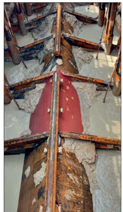
The hopper EcoShield test patch after 10 months of active duty is in excellent condition.
