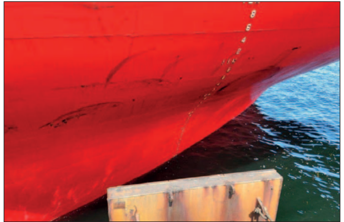
Photos of the Umiak I at Long Harbour in July 2023 showing the condition of the Ecospeed Ice hull coating after two years of plowing through heavy ice. (Photos courtesy Craig Verge, Ship Superintendent.)
