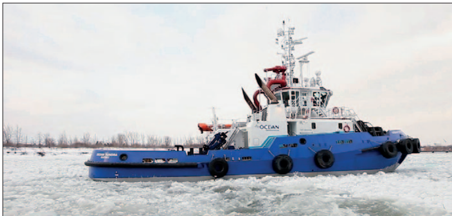
As with all Groupe Océan’s ice-going tugs, the Ocean Tundra is protected with Ecospeed Ice.
