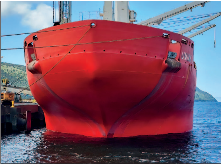
Umiak I two years after Ecospeed Ice application, the hull coating still completely intact with no ice damage whatsoever.
