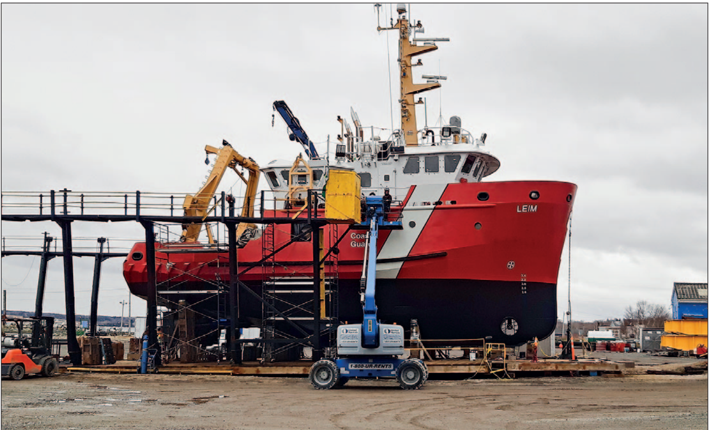
Canadian Coastguard vessel Leim just coated with Ecospeed Ice.
