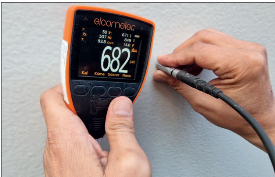
Measuring the thickness of the first layer.
