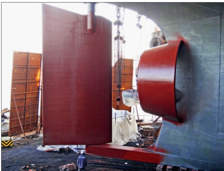
Rudder and nozzle of the Pleiades ship Xanthos with freshly applied Ecospeed. Pleiades Shipping Agents S.A. are a long term repeat customer of Subsea Industries and Bogdanos.
