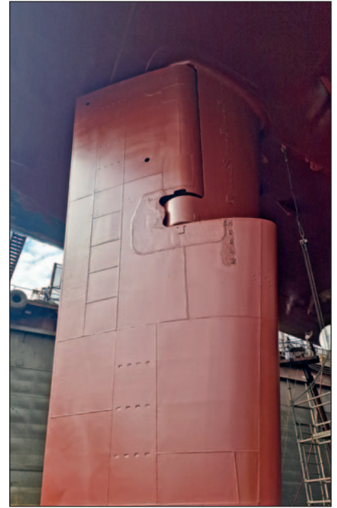
No cathodic protection is needed on rudders
