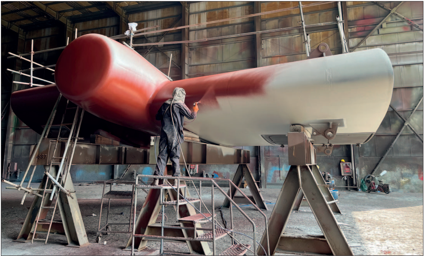
Ecoshield can be applied at the block stage, prior to installation of a rudder.
