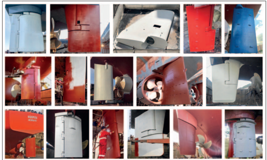
Many major shipping companies turn to Ecoshield to protect the rudders of their ships. Many hundreds of rudders have been coated successfully in the last 20 years. It has put an end to cavitation erosion.
