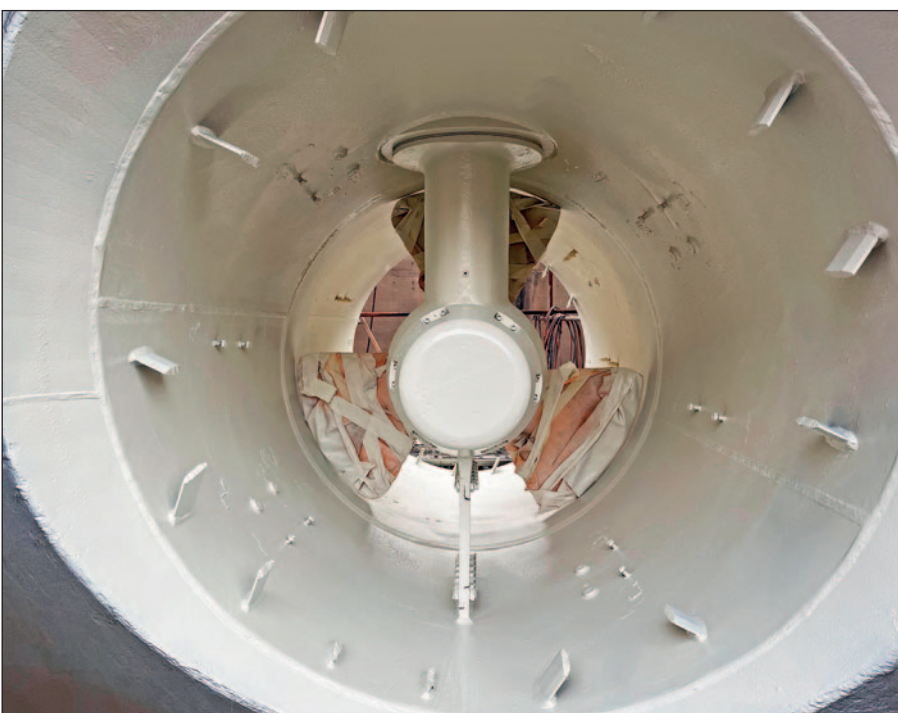
All running gear, including thruster tunnels, can be protected with Ecoshield.
