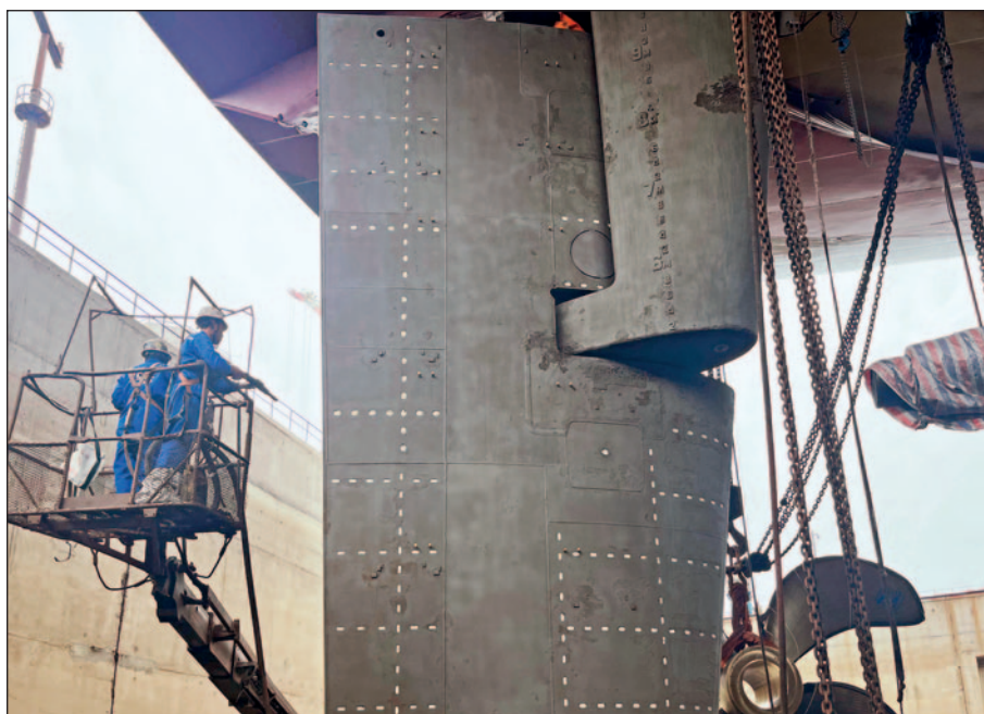
Rudder after surface preparation.
