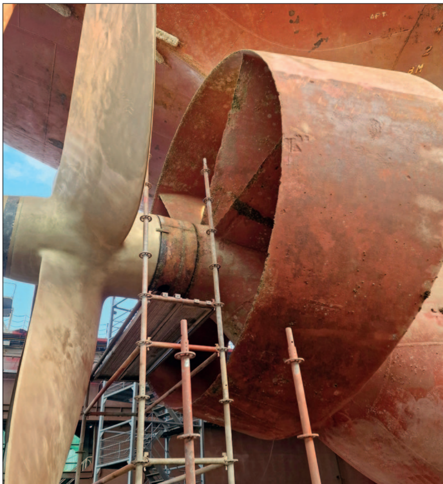
Cavitation damage on energy saving device prior to Ecoshield application.
