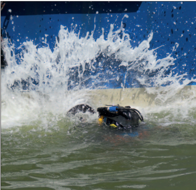
When divers clean an Ecospeed hull, there is no paint loss and no toxic plumes are created.
