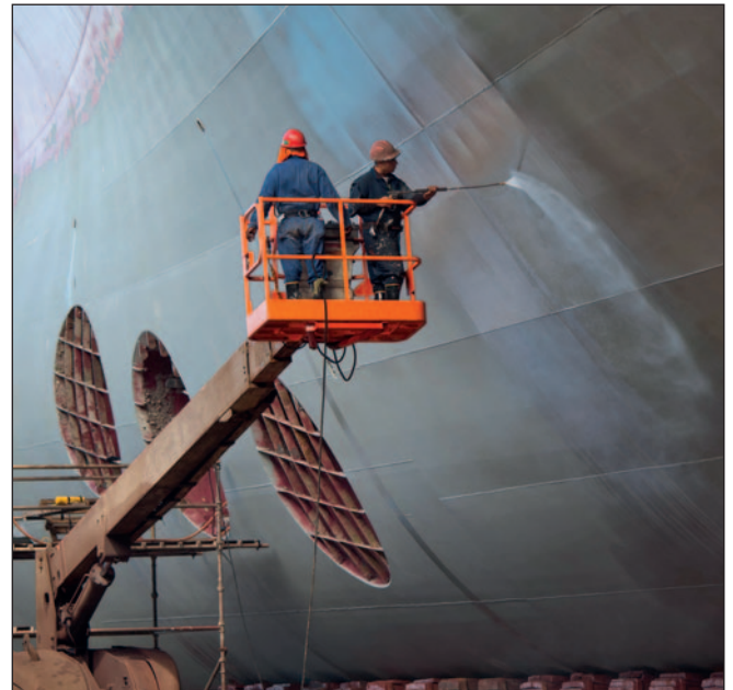
The coating can be quickly washed in drydock with high pressure tools.
