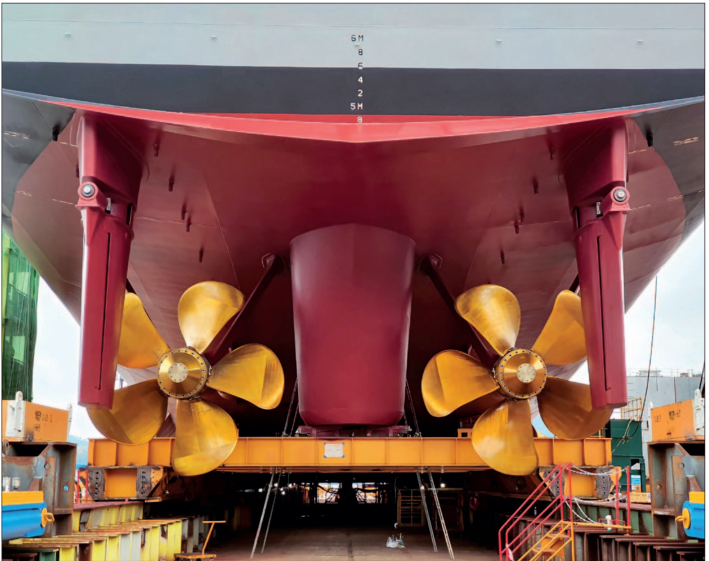
Rudders of ROK Navy MARS tanker designed by ECOTEC and protected with Ecoshield.
