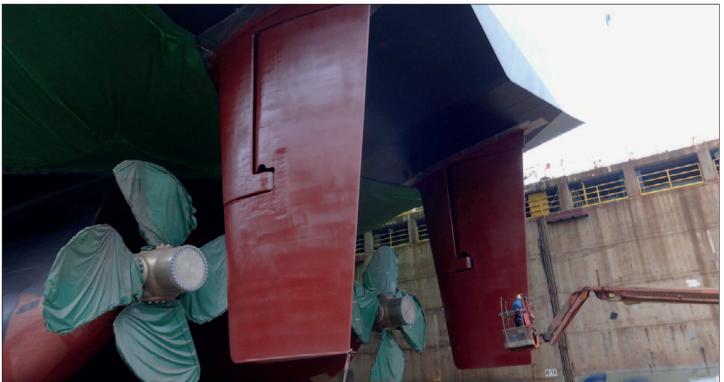
Rudders of one of four UK Royal Navy MARS tankers designed by ECOTEC and coated with Ecoshield coating for permanent protection from cavitation erosion and corrosion.
