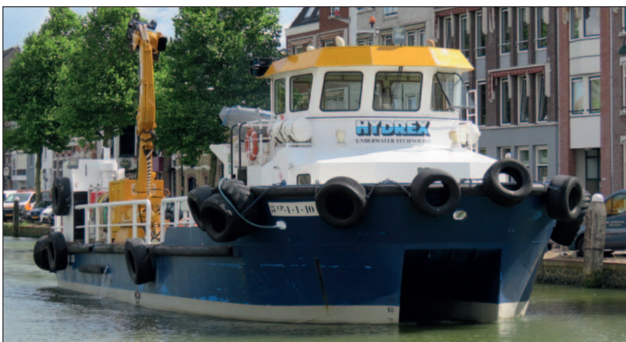
This dive support vessel was coated with Ecospeed 14 years ago. It can be cleaned effortlessly and legally in harbours, such as the Port of Rotterdam, which have banned the underwater hull cleaning of conventional coatings.
