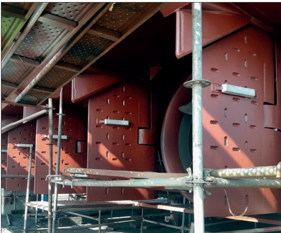
The rudders of the newbuild icebreaking tug Antarctic protected for life with Ecoshield.
