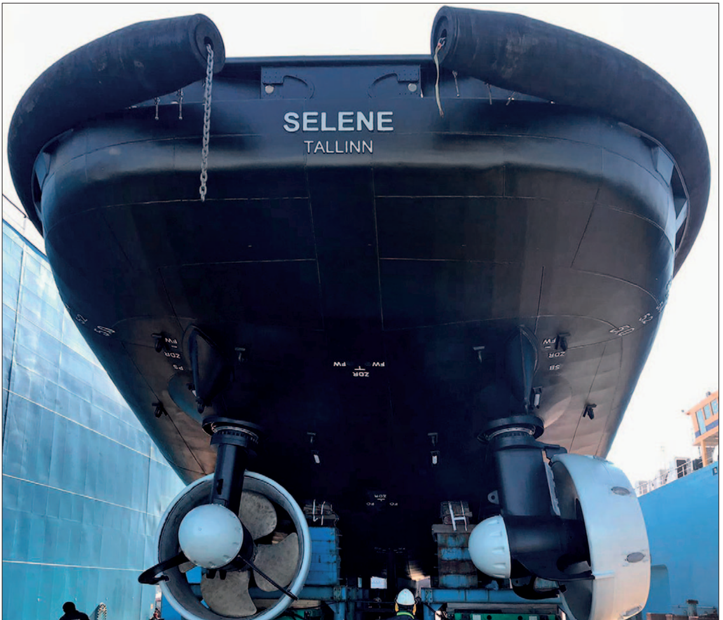
Alfons Håkans Selene newbuild ice class tug coated from gunwale to keel with Ecospeed preparing for launch.
