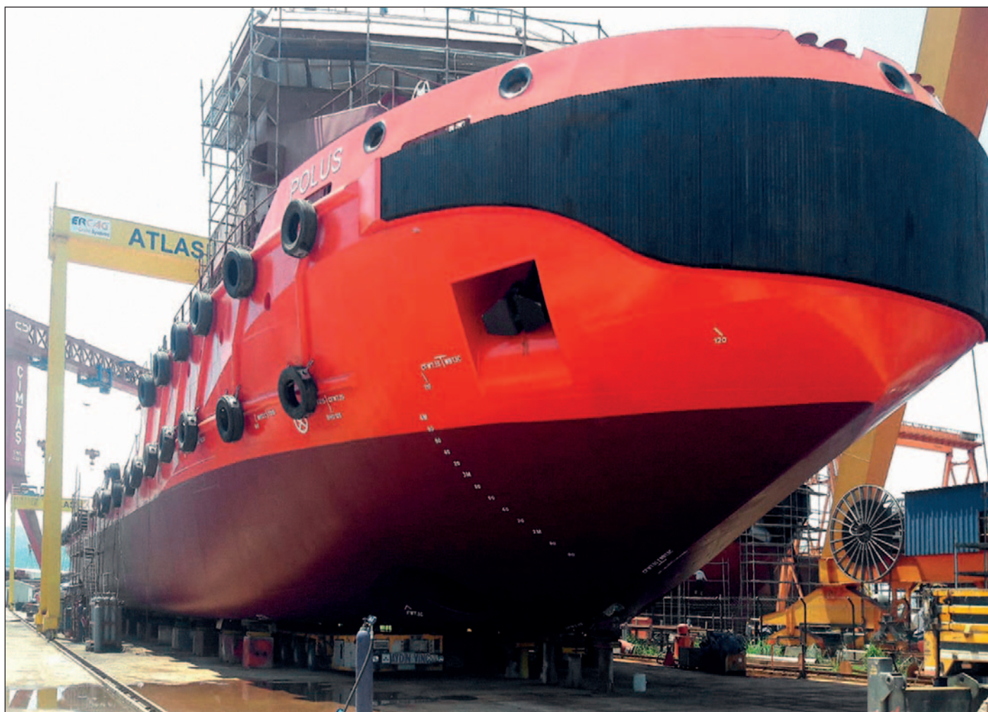
Ark Shipping's Polus nearing completion at the Atlas shipyard in Turkey. The underwater hull (dark red) is newly applied Ecospeed.
