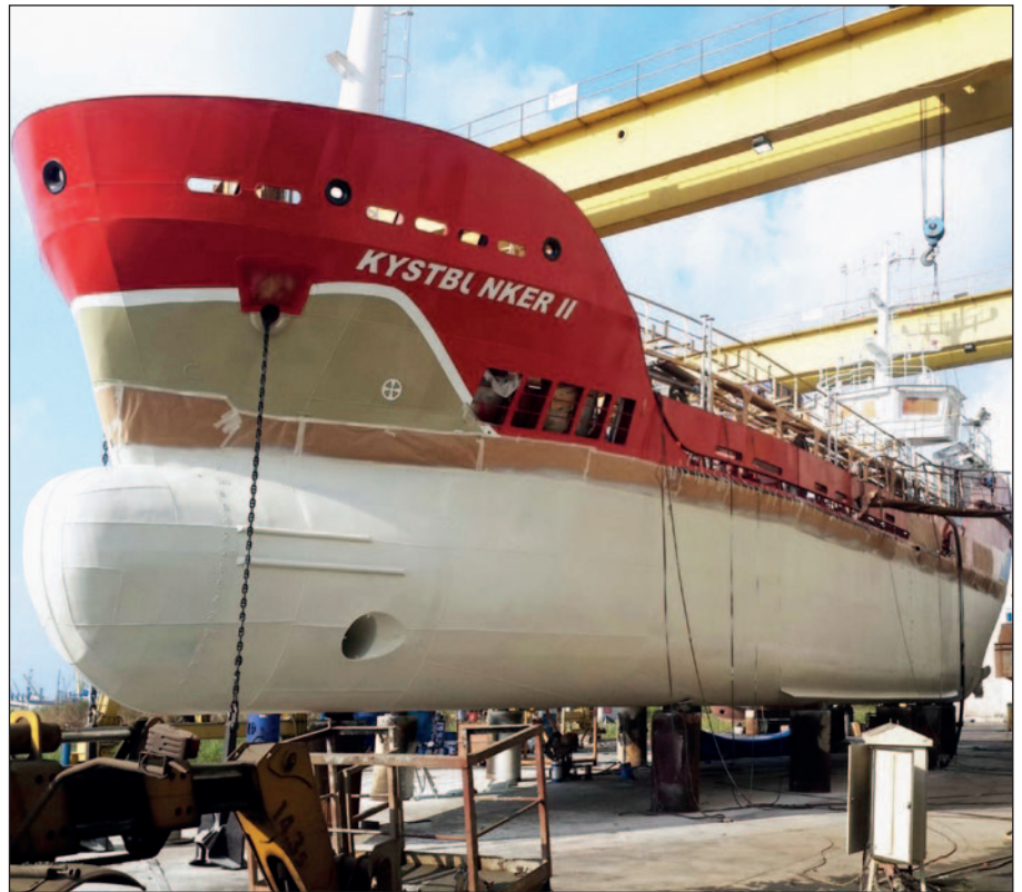
The near complete newbuild M/V Kystbunker II at Akdeniz shipyard after the first coat of Ecospeed has been applied.
