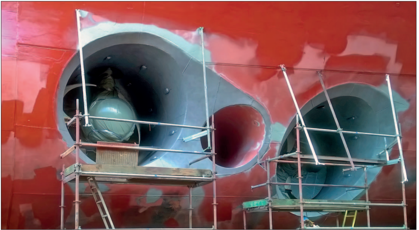
Per was Subsea Industries' agent and inspector of the Ecoshield application on the thruster tunnels of the Finnlines Ro-Pax MS Finnfellow at Turku Repair Yard, Naantali, Finland in 2016.
