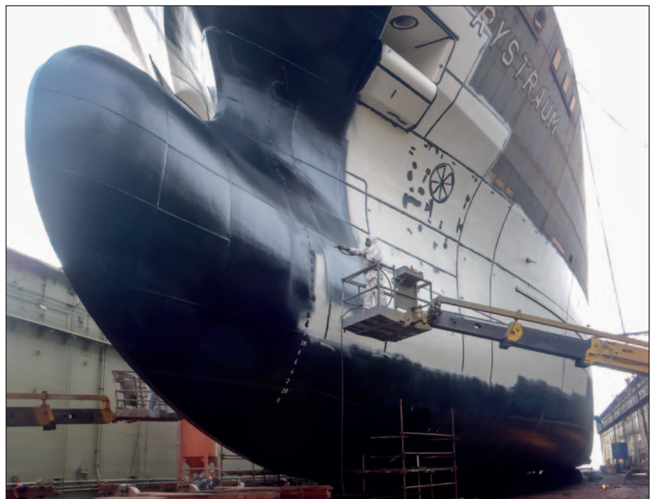
The second coat of Ecospeed being applied to the Rystraum at the 3.Maj shipyard.
