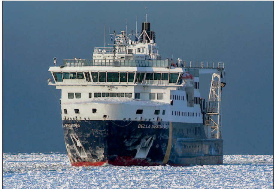
The Bella Desgagnés protected with Ecospeed ice-abrasion resistant coating sails in ice off Quebec.
