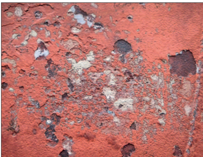
It is impossible to repair an antifouling coating that has degraded over time and restore the hull to a smooth finish.
