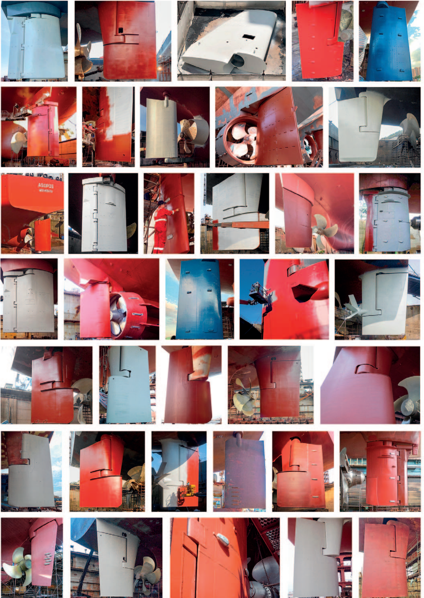
Well over 1000 Ecoshield applications to rudders and running gear testify to the coating's effectiveness in protecting these underwater ship parts from cavitation erosion.
