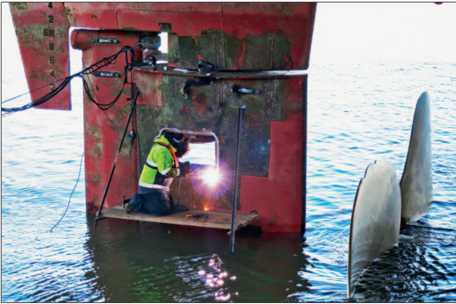
Lack of proper protection of the rudder can lead to serious damage and sometimes the need for emergency repairs out of drydock.
