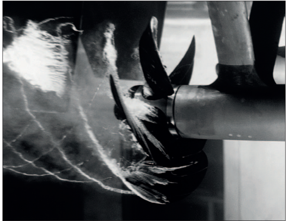
Cavitation from a propeller. Photo: U.S. Navy, Public domain, via Wikimedia Commons.
