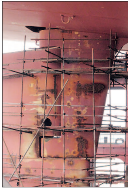
A. The rudder of a large container ship after 5 years of sailing with only conventional hull coating for protection.
