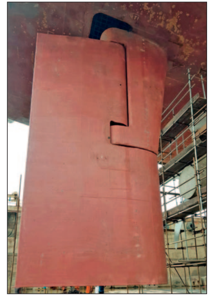
B. The same rudder after 10 years of sailing with Ecoshield. The coating has not been replaced. Seen here after being washed off in drydock.
