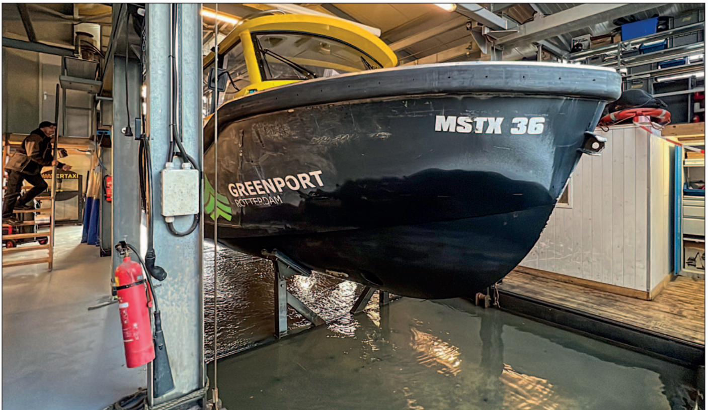
While in service, the taxi's hull is rapidly pressure washed every month to remove slime and any other fouling that has accumulated. This is done at the Watertaxi Rotterdam Kop van Zuid headquarters and maintenance facility.
