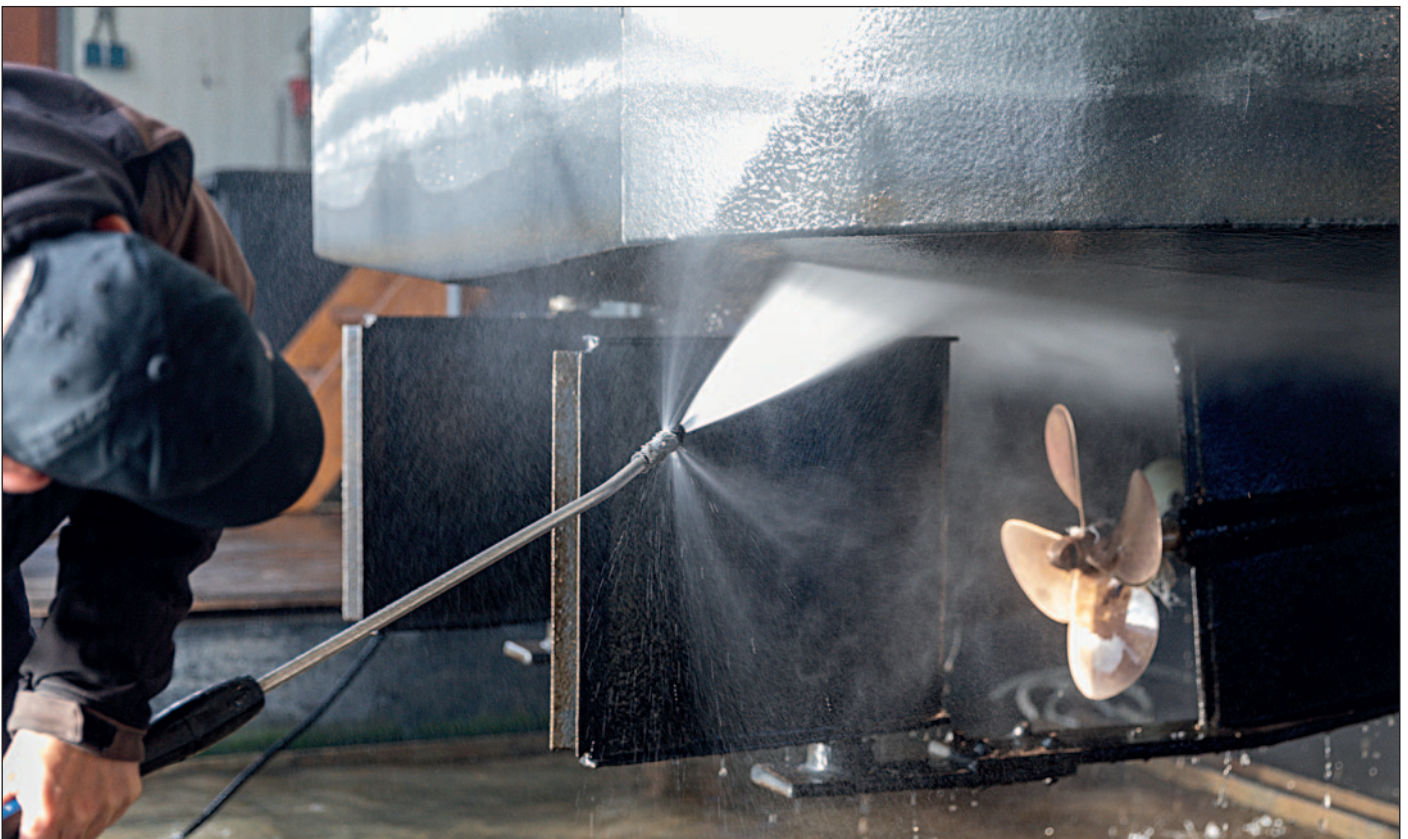
Pressure washing the Ecospeed coated hull is quick and simple and does not damage the coating or pollute the environment.
