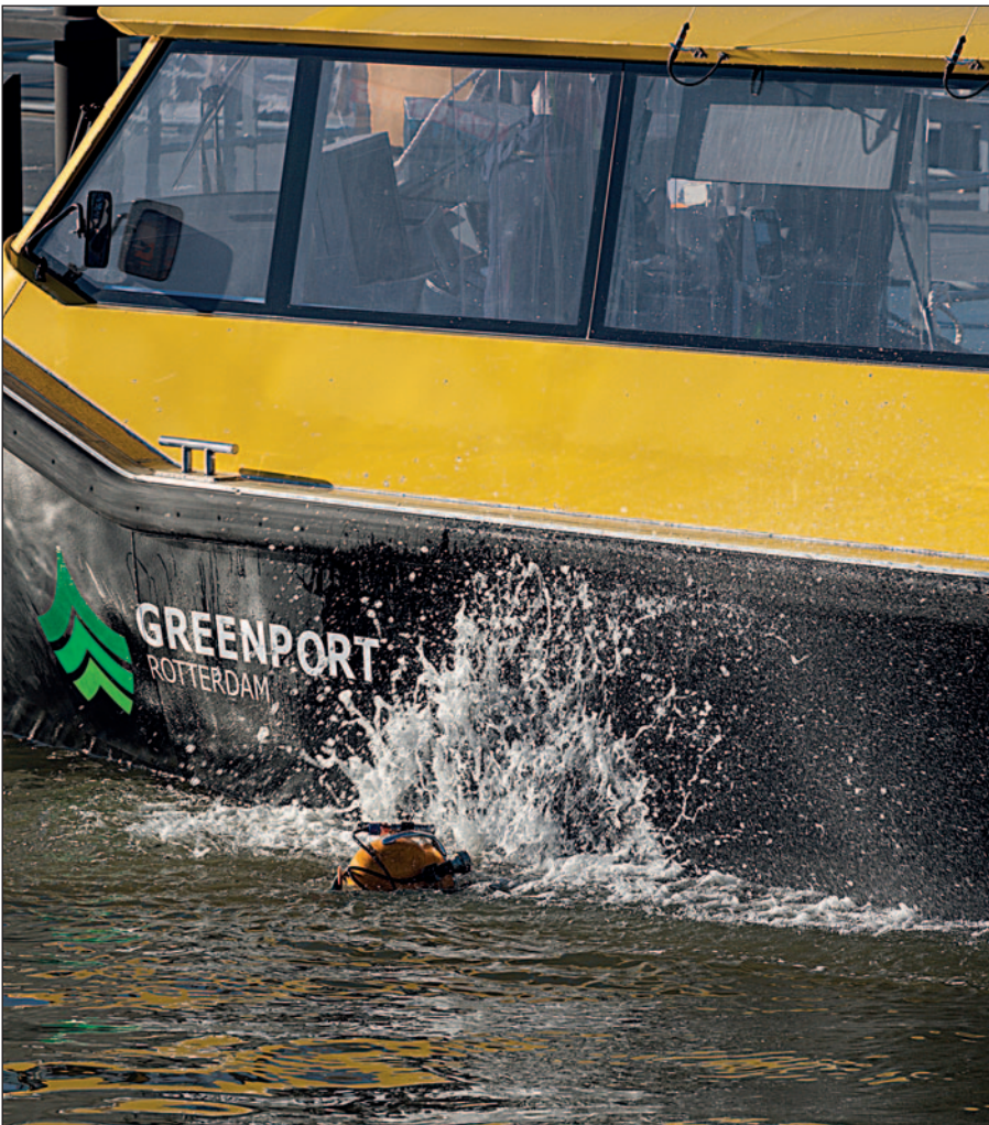
Conditioning the hull by a diver using our underwater cleaning tools results in improved hydrodynamic performance.
