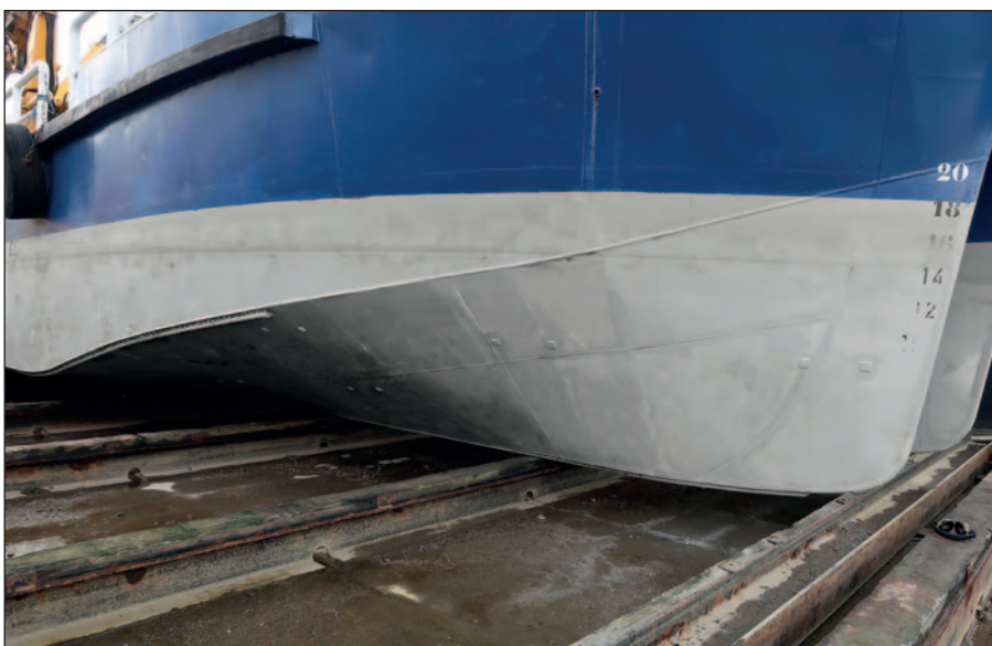
The hull of a Hydrex workboat sailing with Ecospeed for 12 years without recoating. Hydrex has the security of knowing that the hulls of its workboats are entirely non-toxic. Keeping them clean is not a problem.
