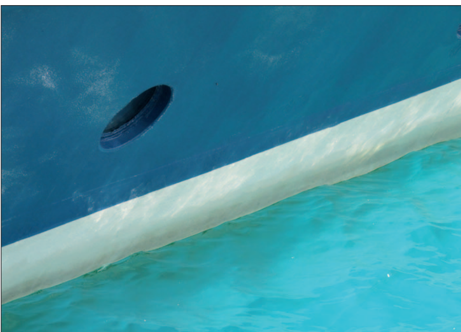
The water line of a cruise ship coated with Ecospeed 12 years before the photo was taken. The coating has not been replaced since first applied. The hull is kept clean by the crew during normal cruise operations.
